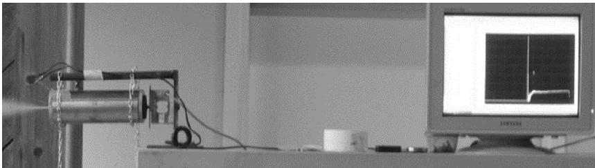
**Figure 3.** Burning MTP rocket engine and thrust curve at the monitor.
