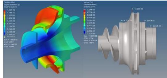
Figure 12 - LOx pump FEA analysis for the SS316L AM material.
