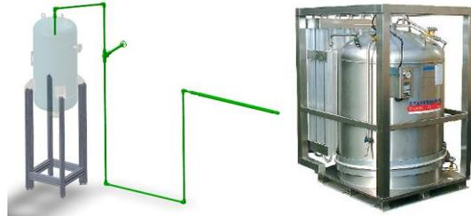
Figure 31 - Tank filling line, highlighted in green.
