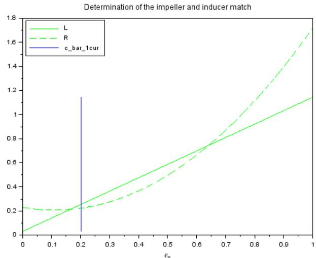
Figure 3 – Left (continuous) axial inducer and right (dashed) centrifugal impeller cavitation characteristics for blades geometry matching.
