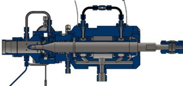
Figure 17 - The final design of the LOx pump.
