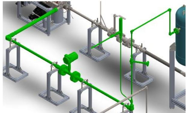
Figure 28 - High-pressure line highlighted in green.
