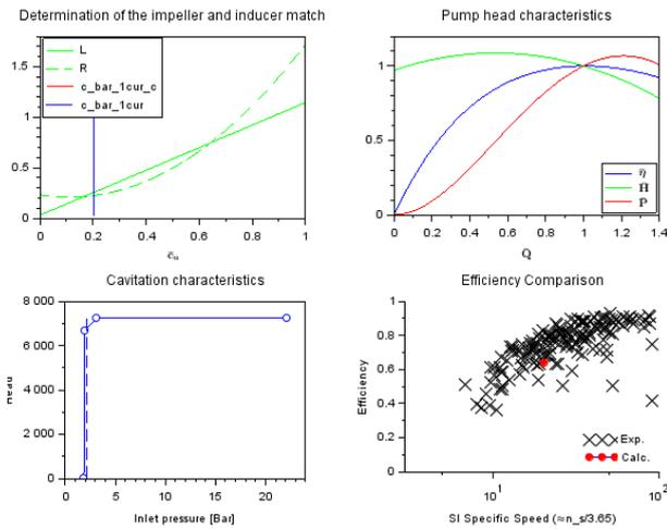
Figure 4 - Plot with some of the outputs from the PUMPCALC code
