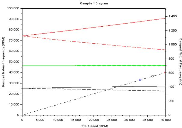
Figure 15 - Campbell's diagram of the first design iteration.
