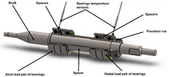
Figure 18 - Bearings architecture for the final design.
