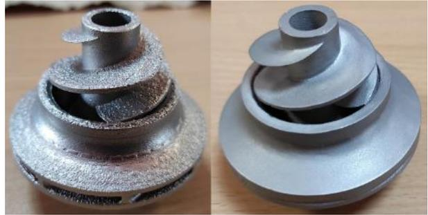
Figure 23 - Left, 50µm layer with open impeller and bead blasted. Right, 20µm layer with closed impeller, bead blasted and tumbling.
