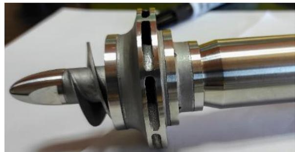
Figure 25 - Pump after machining at the shaft with the pump nut installed.
