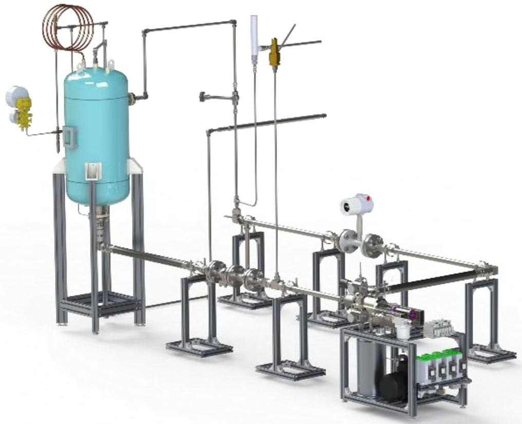
Figure 32 - Cryogenic pump test bench
