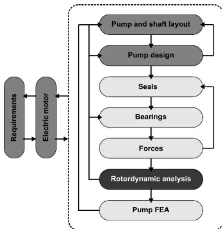
Figure 1 - Pump design flow chart, adapted from [2].
