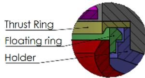
Figure 9 – Floating ring main seal schematic.
