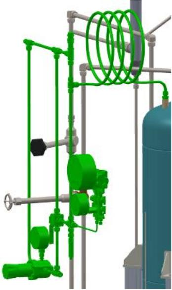
Figure 30 - Tank pressure and level control system highlighted in green.
