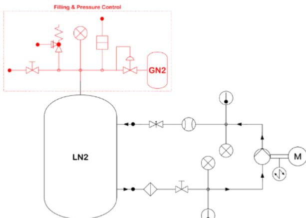
Figure 26 - Cryogenic test bench piping and instrumentation diagram.
