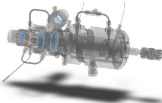
Figure 11 - Cryogenic static seals of the pump assembly and flanges.
