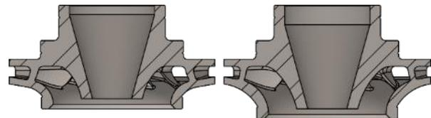
Figure 8 – A cut view of a LOx pump as originally designed (left) and optimized for AM (right).
