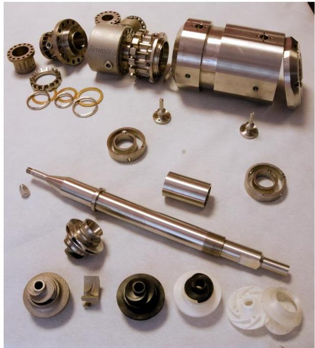
Figure 24 – Manufactured components of the LOx pump.
