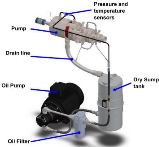
Figure 21 - Lubrication system schematic.
