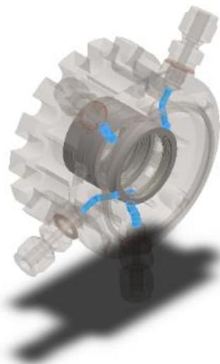
Figure 10 – Shaft seals with the inlet and outlets of the two cavities purged by GN2.
