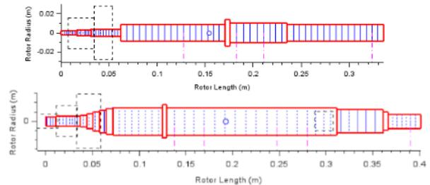
Figure 13 - Example of meshes for the first and one of the latest iterations for the shaft design using the ROTORDYN mesh.
