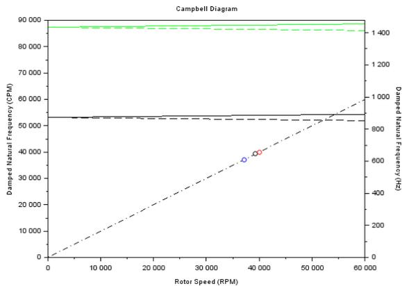
Figure 16 - Campbell's Diagram for the final design of the shaft and bearings.
