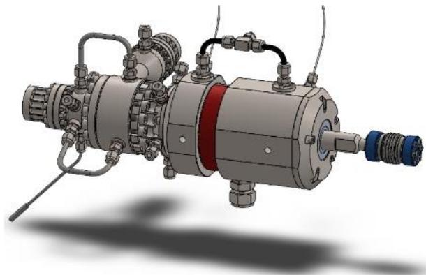
Figure 22 - View of the final design of the LOx pump assembly.
