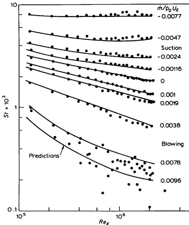
Figure 11 Predicted and measured variation with length Reynolds number of Stanton number for heat transfer to a porous flat plate with low temperature ratio and various degrees of suction and blowing. (Data from Moffat and Kays, 1968). (Taken from references 154)
