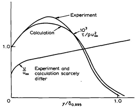
Figure 4 Equilibrium boundary layer with  $u_\infty \propto x^{-0.15}$ . Calculations by Bradshaw *et al*. (Figure taken from reference 4)
