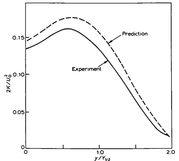
Figure 14 Turbulence kinetic energy ( $X/h = 70$ ). (Plane-jet data from Bradbury, 1965). (Taken from reference 154)
