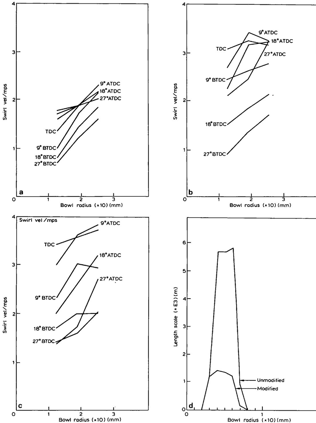
Figure 21 Swirl velocity (taken from reference 169). (a) Standard  $k \sim \epsilon$ ; (b) modified  $k \sim \epsilon$ ; (c) measurements (reference 170); (d) length scale at TDC. mps is mean piston speed ( $8.19 \text{ m s}^{-1}$ )
