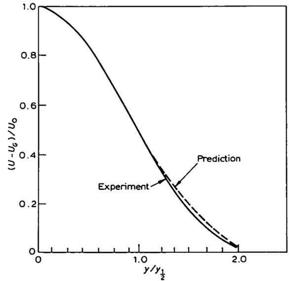
Figure 12 Axial mean velocity ( $X/h = 70$ ). (Plane-jet data from Bradbury, 1965). (Taken from reference 154)
