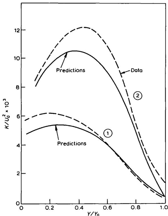
Figure 9 Predicted and measured turbulence energy on a flat plate with (1) mild and (2) severe pressure gradients. (Data from Bradshaw, 1965). (Taken from reference 154)
