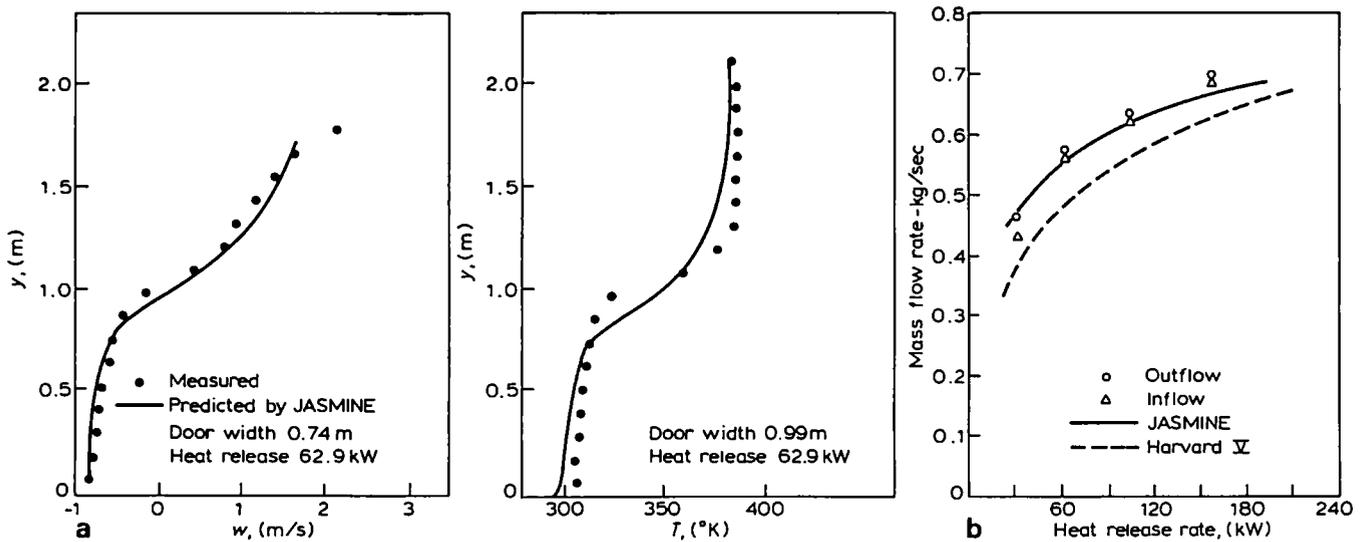
Figure 17 Smoke flow in 3D enclosures. (Taken from reference 35). (a) doorway velocity and corner temperature profiles; (b) comparison of Steckler's data with predictions of field and zone models
