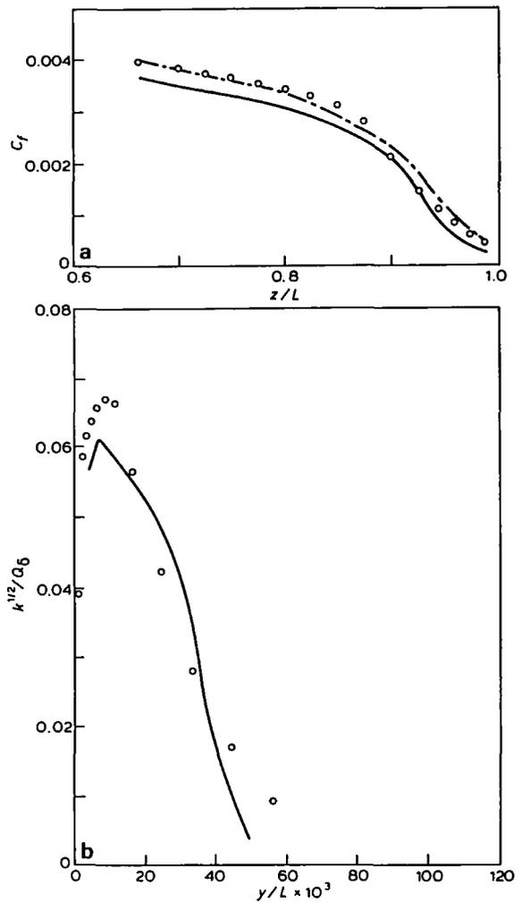
Figure 20 Flow around bodies of revolution. (Taken from reference 166).  $Q_\delta$  is total velocity at boundary layer edge. (a) viscous-flow, full-body: distribution of skin friction coefficient along hull (b) viscous-flow, half-body: lateral variation of turbulent kinetic energy at  $z/L = 0.96$ . (ooo), predictions; (—), Patel experiment (reference 206); (- · - · -) Thompson (206)
