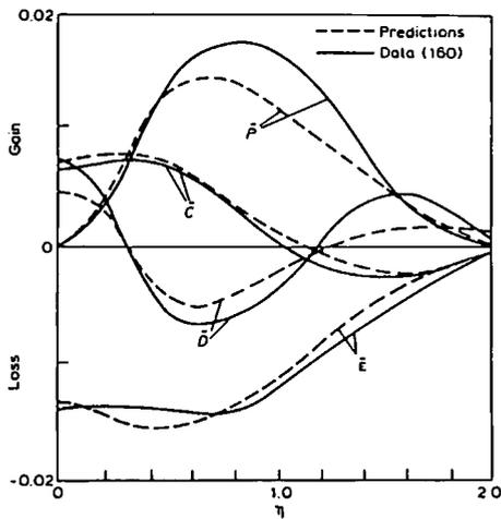
Figure 15 Plane jet, turbulent-kinetic-energy balances in self-similar region. (Taken from reference 155)
