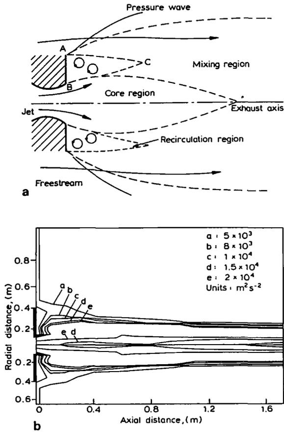
Figure 19 Flow and combustion in base-wall region of a rocket exhaust plume. (Taken from reference 204). (a) flow field around missile base wall; (b) contours of turbulence kinetic energy ( $\text{m}^2\text{s}^{-2}$ ) for conditions of case 2, base wall present and free stream Mach number  $M_U = 2.9$
