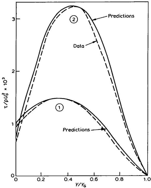
Figure 10 Predicted and measured shear stress on a flat plate with (1) mild and (2) severe pressure gradients. (Data from Bradshaw, 1965). (Taken from reference 154)
