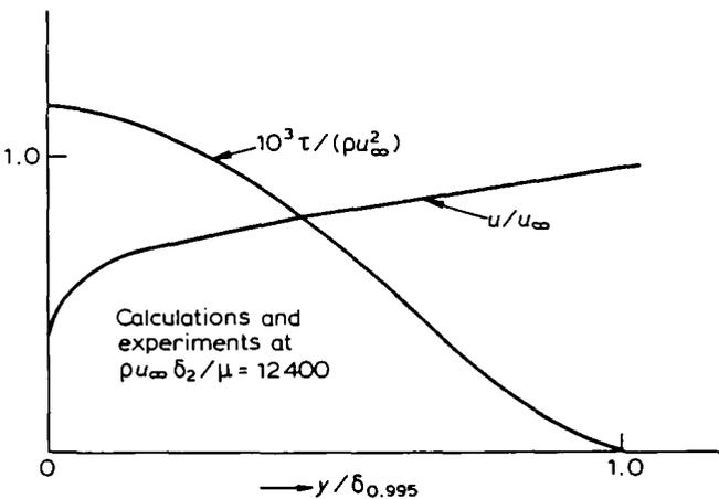
Figure 3 Flow past a flat plate with uniform  $u_\infty$ . Calculations by Bradshaw *et al*. (Figure taken from reference 4)
