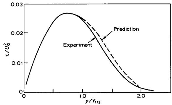
Figure 13 Shear stress ( $X/h = 70$ ). (Plane-jet data from Bradbury, 1965). (Taken from reference 154)
