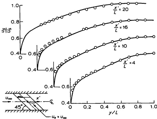
Figure 1 Predictions of a swept-wing boundary using equation (23) (O), experiments (reference 51); (—), calculations. (Taken from reference 1)
