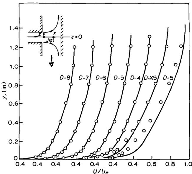
Figure 2 Predictions of a laterally diverging boundary layer using equation (23). (O), experiments (reference 52); (—), calculations. (Taken from reference 1)
