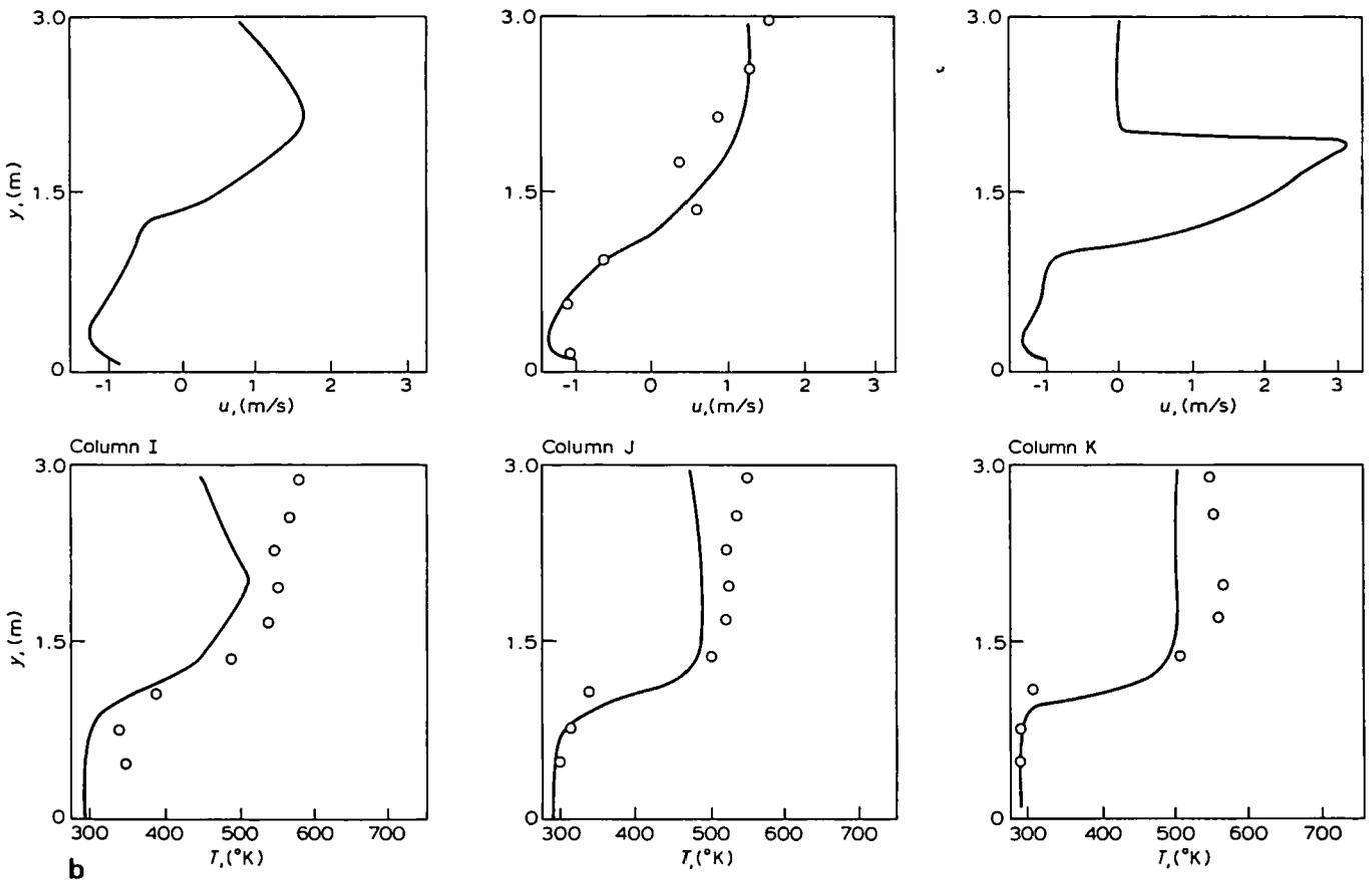
Figure 18 Smoke flow in enclosures (Taken from reference 205). (a) Plan of mall showing instrumentation; (b) predicted and measured velocity and temperature profiles for  $D = 1$  m
