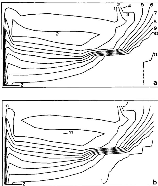
Figure 16 3D fires in enclosures (Taken from reference 36). (a) distribution of oxidant (10 contours in range 0.44-1.0); (b) distribution of combustion products (10 contours in range 0.001-0.55); (c) comparison of velocity profiles at door (symmetry plane). (—), predictions; (---), experiment; (d) comparison of temperature profiles at door (symmetry plane), (—), predictions; (---), experiment
