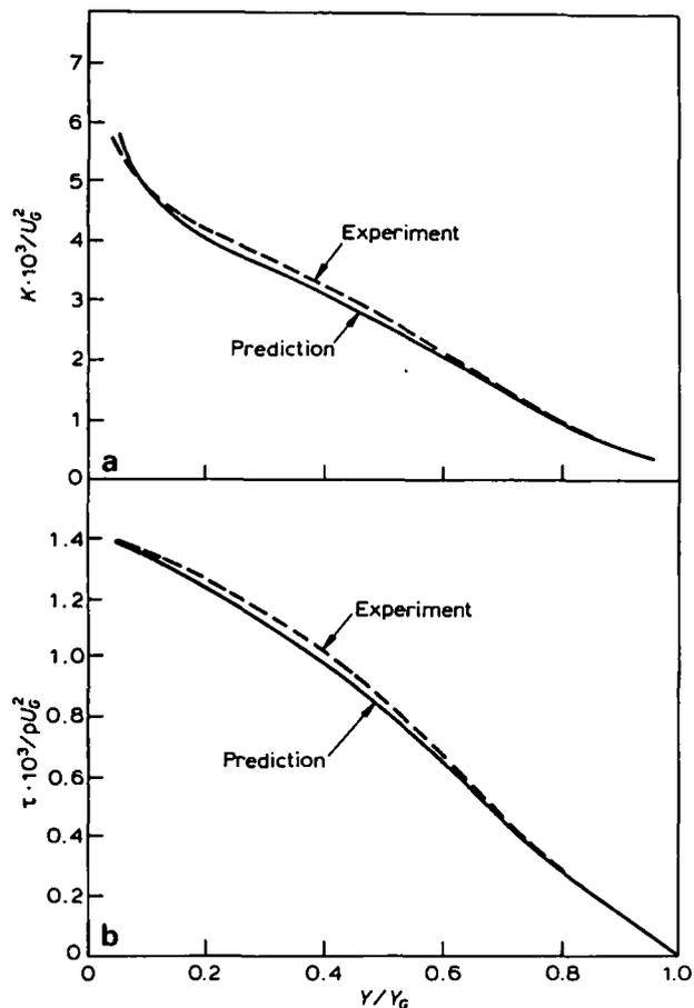
Figure 8 Distributions on flat plate of (a) turbulence kinetic energy; (b) Reynolds shear stress. (Experimental data from Klebanoff, 1984). (Taken from reference 154)
