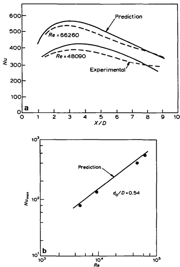
Figure 7 (a) Nusselt number distribution for  $d_0/D = 0.54$  (Pipe-expansion data of Zemanick and Dougall, 1970). (Taken from reference 154). (b) Variation of maximum Nusselt number with Reynolds number  $d_0/D = 0.54$ . (Pipe-expansion data from Zemanick and Dougall 1970). (Taken from reference 154)
