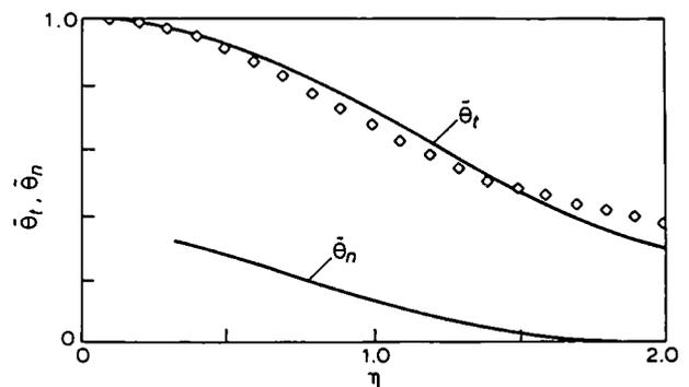
Figure 23 Plane turbulent wake. Comparison of measured and predicted similarity profiles of conditional temperatures (taken from reference 29).  $\bar{\theta} \equiv (T - T_\infty) / \Delta T_m$  where  $\Delta T_m$  is maximum temperature excess. (—), predictions; ( $\circ$ ), experiments, reference 203. Subscripts,  $t$  = turbulence,  $n$  = nonturbulence
