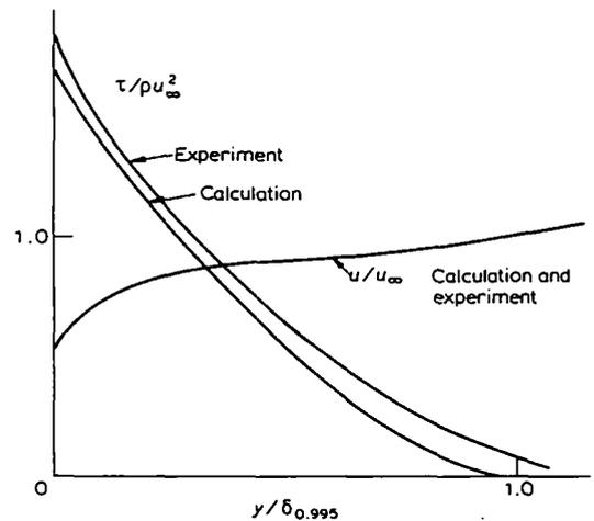
Figure 5 Equilibrium boundary layer in favourable pressure gradient. Calculations by Bradshaw. (Figure taken from reference 4)
