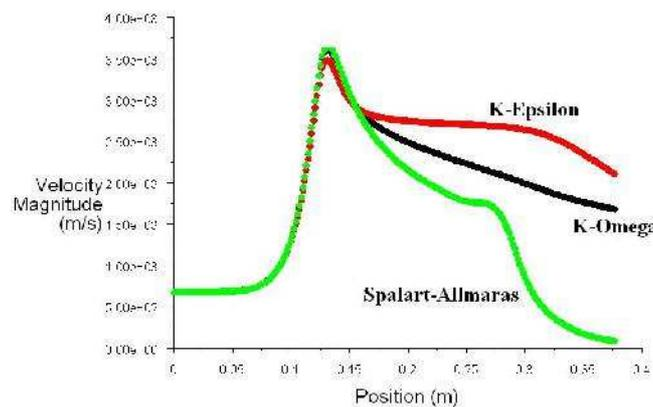
Fig 6, Velocity distribution plot at Mach no-2
