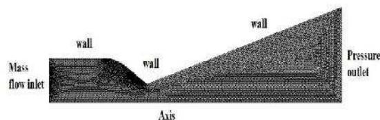
Fig 2, Computational Model of C-D nozzle
