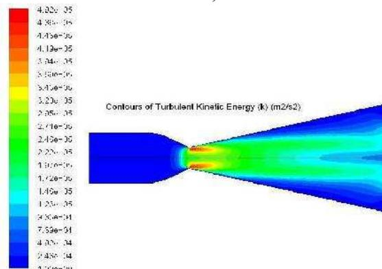
Fig 4, Turbulence kinetic energy contours for K-Omega model (Mach no-2)
