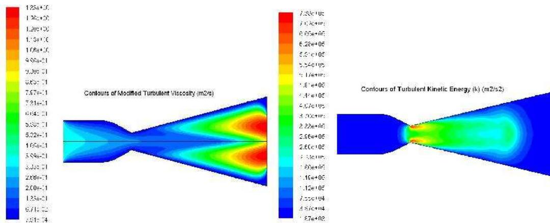
Fig 3, Turbulence kinetic energy contours for spalart-Allmaras model and K-Epsilon model (Mach no-2)
