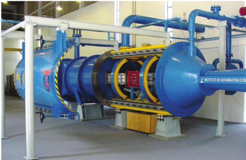
Figure 4. Part of the aerodynamic circuit of the TTP showing the opened plenum chamber.
