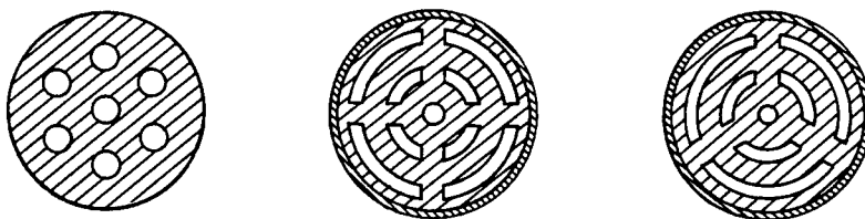
Figure 25.—Typical multiperforated grain shapes.
