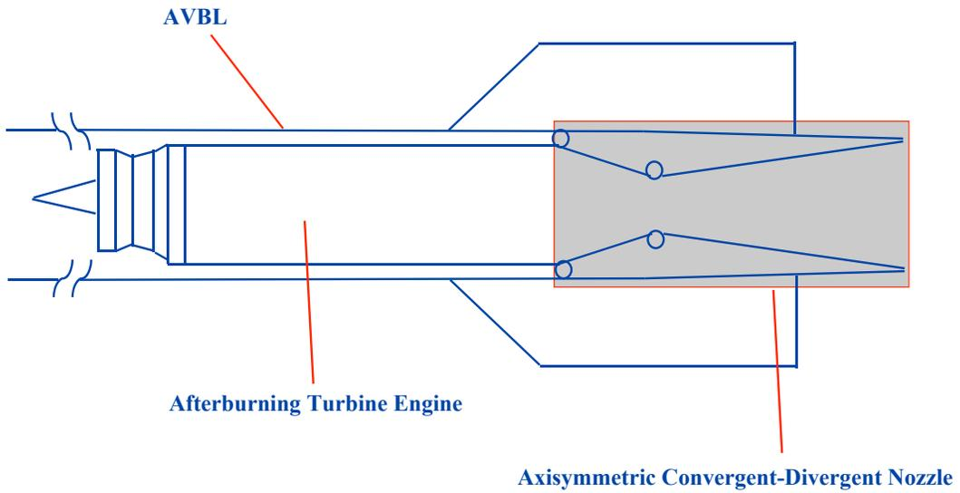
**Fig. 2. Schematic of the AVBL engine/nozzle integration.**
