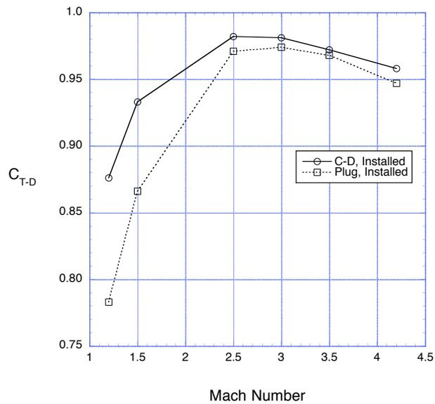
**Fig. 13. Comparison of installed performance for the C-D and plug nozzles.**
