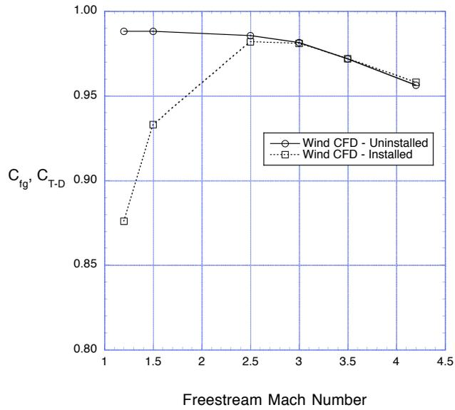
Fig. 7. Comparison of uninstalled and installed performance for the C-D nozzle.
