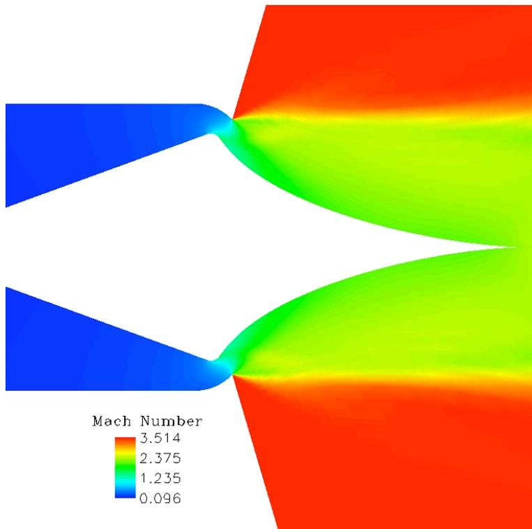
**Fig. 10.** Mach number contours for inviscid nozzle calculation at design nozzle pressure ratio.
