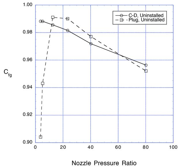
**Fig. 12. Comparison of uninstalled performance for the C-D and plug nozzles.**
