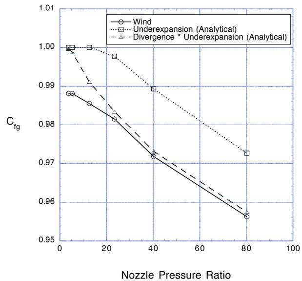
**Fig. 5. Uninstalled performance for the axisymmetric C-D nozzle.**
