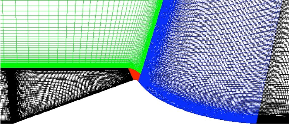
**Fig. 9.** Computational grid for isentropic plug nozzle for Mach 4.2 flight configuration (region near nozzle shown).
