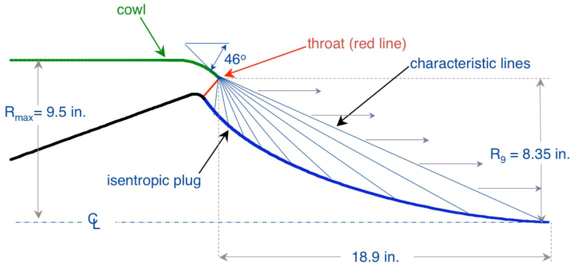
Fig. 8. Isentropic plug nozzle schematic.
