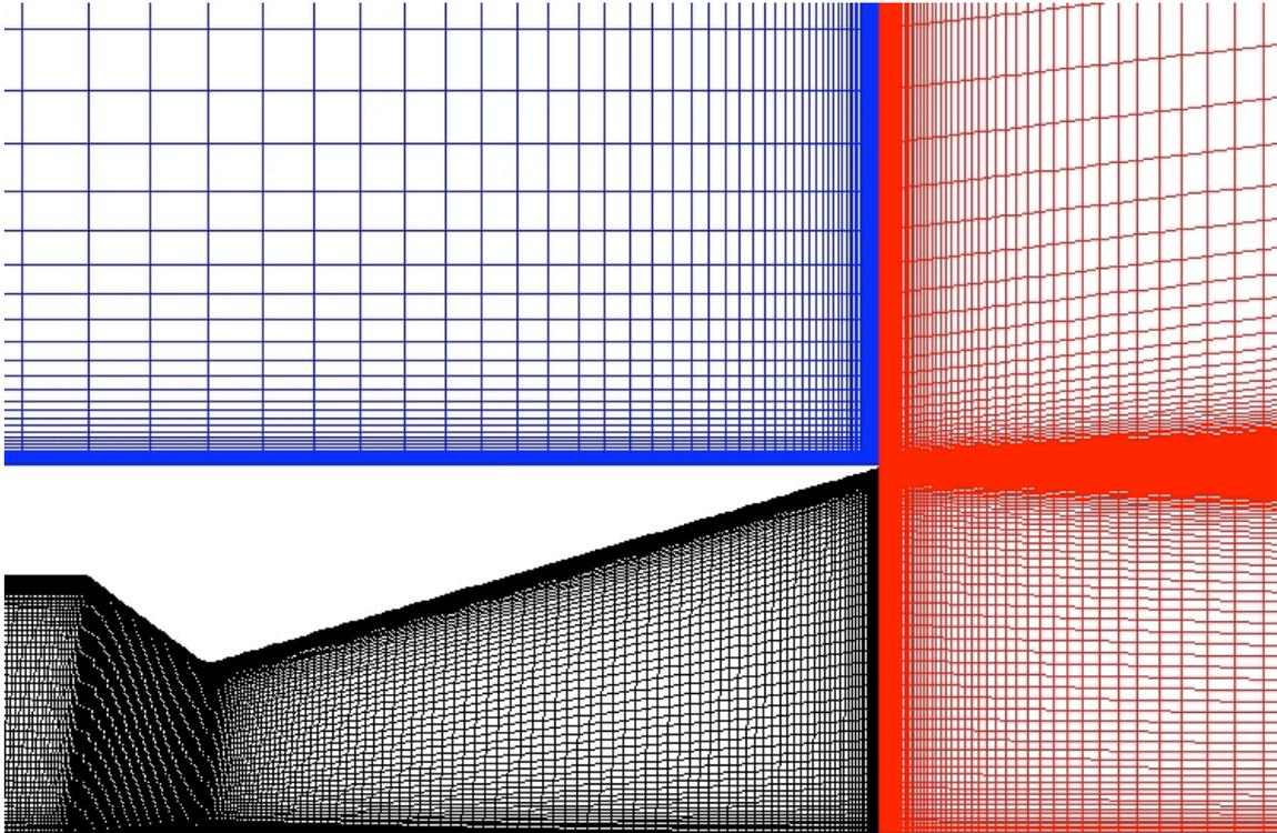
**Fig. 3. Computational grid for axisymmetric C-D nozzle for Mach 4.2 flight configuration (region near nozzle shown).**
