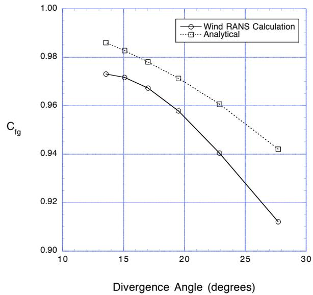
**Fig. 4. Variation of internal nozzle performance with divergence angle.**
