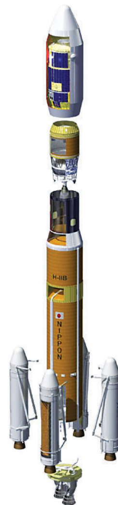
Fig. 5 Schematic of newly developing H-IIB launch vehicle. The clustered LE-7A are installed as the first stage engine.
