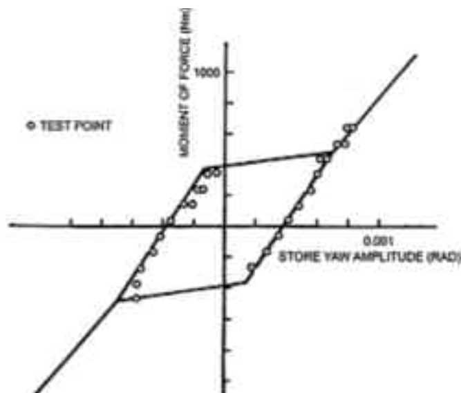
Fig. 2. Store yaw amplitude vs. force moment for the F-111 aircraft
