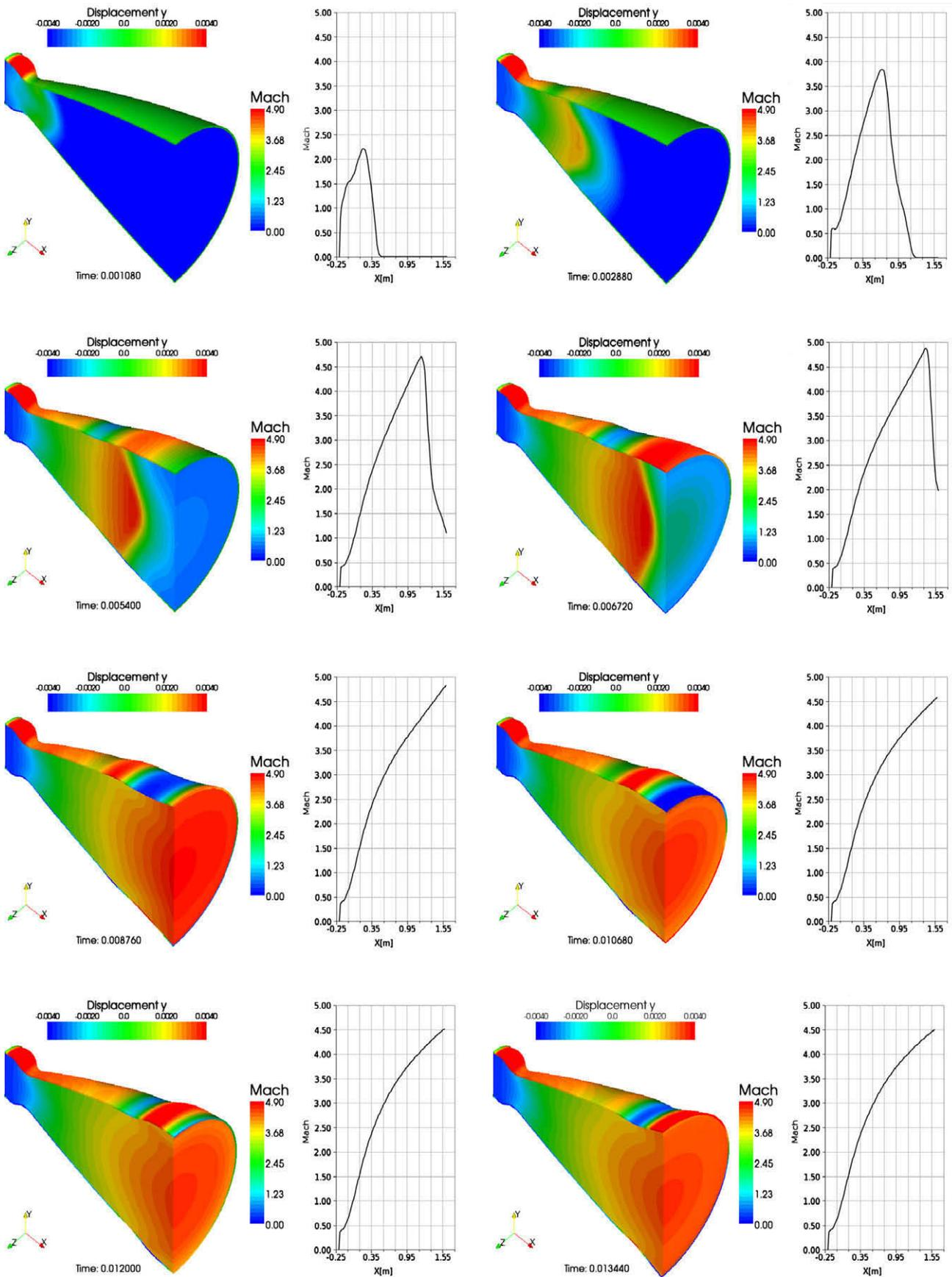
Fig. 12. Ignition process of the rocket engine.
