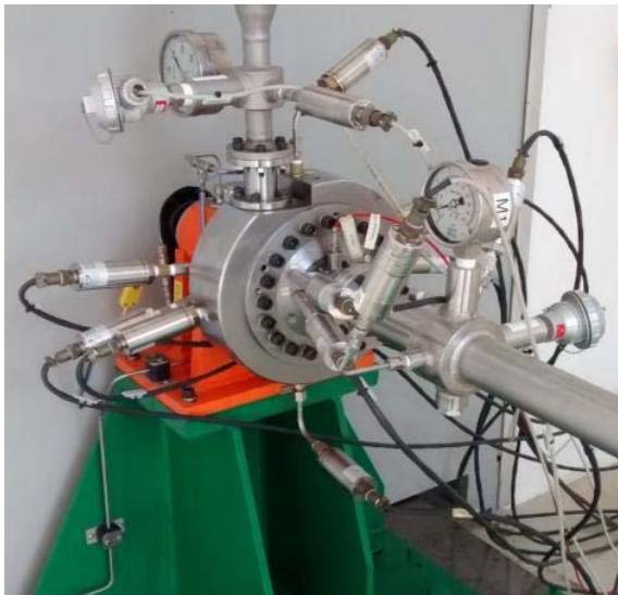
Figure 13: LOx pump development model installed in the test stand.
