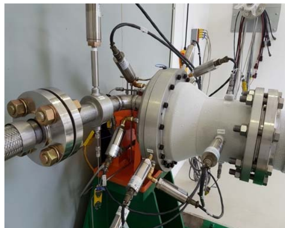
Figure 15: Turbine predevelopment model installed in the test stand
