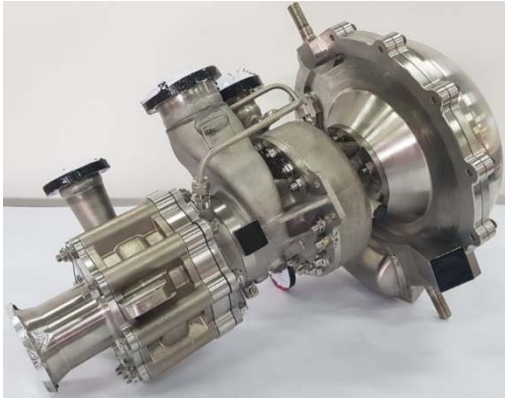
Figure 12: Turbopump manufacturing demonstrator
