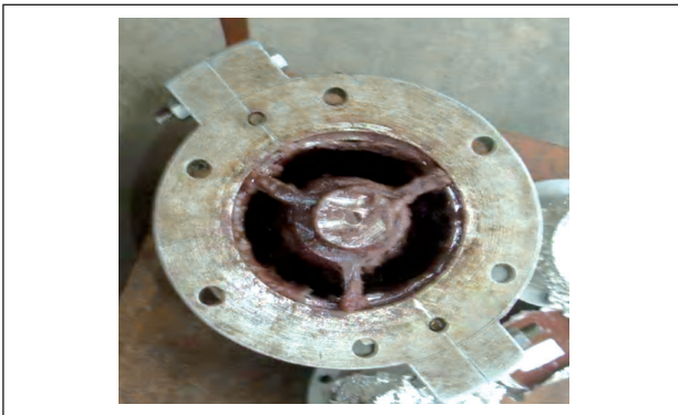
Figure 6. Casting mould with collapsible mandrel after casting.
