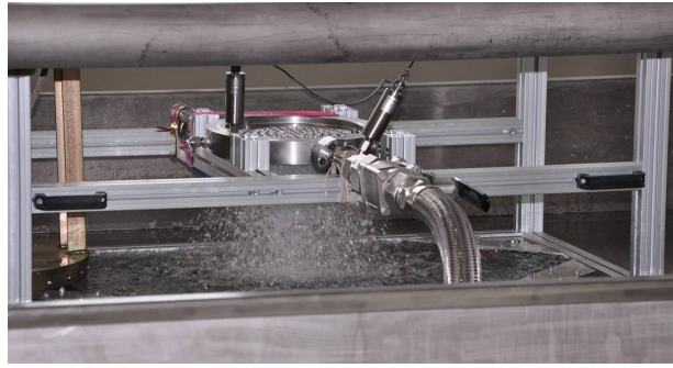
(b) L75 PDM 1 injector head flow tests
