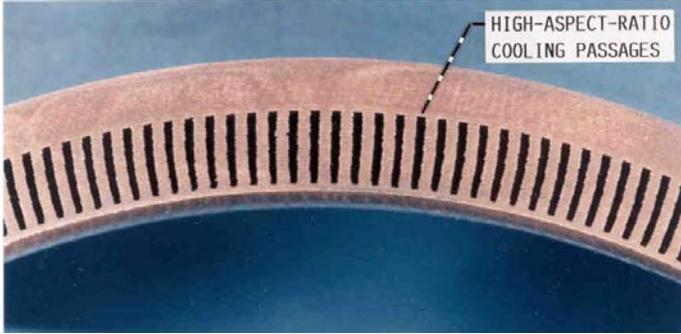
Figure 3: Cross-section of a high-aspect-ratio cooling passage
