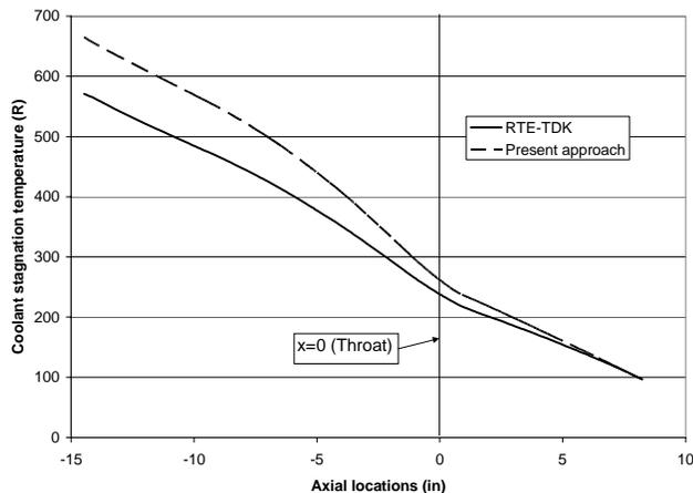
Figure 8: Comparison coolant temperature of the SSME based on the present approach and that of RTE-TDK
