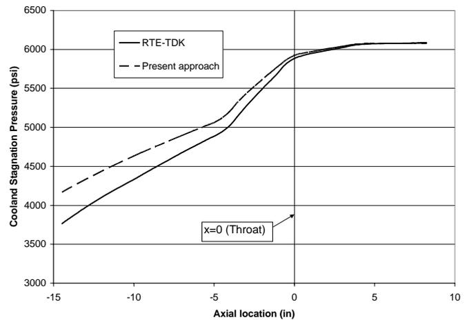
Figure 9: Comparison coolant pressure of the SSME based on the present approach and that of RTE-TDK
