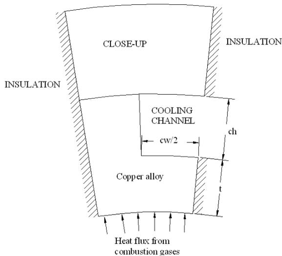
Figure 4: Configuration of one cell cooling channel
