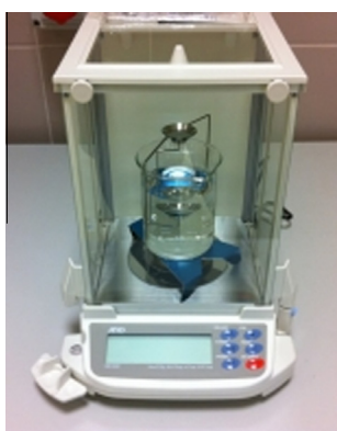
Fig. 17. The instrument used in measurement of density of the solid propellant samples with the degree of accuracy as 0.0001.
