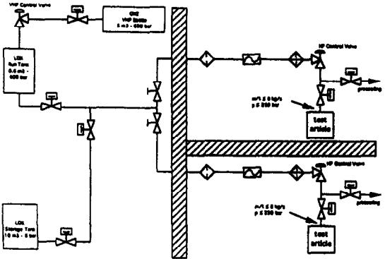
Fig. 2 Simplified flow diagram of LO<sub>2</sub>-supply system at P8.
