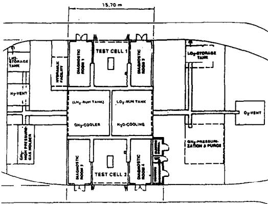
Fig. 1 General arrangement of P8 test bench for LO<sub>2</sub>/GH<sub>2</sub>-high pressure combustion.
