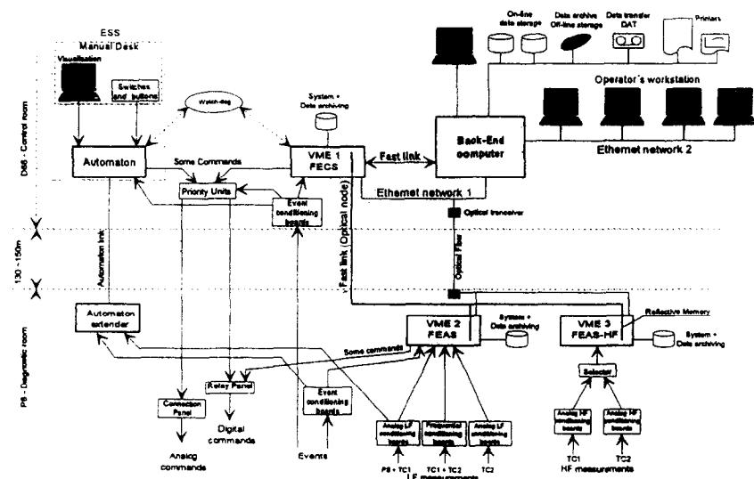
Fig. 4 MCC-system hardware architecture of P8.
