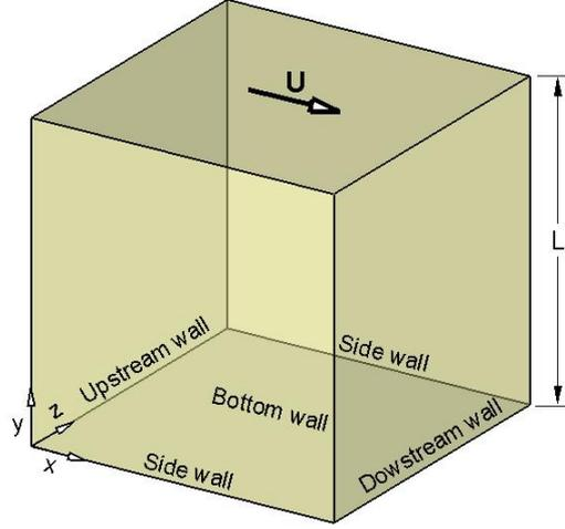
Figure 1. Lid-driven cubical cavity geometry.
