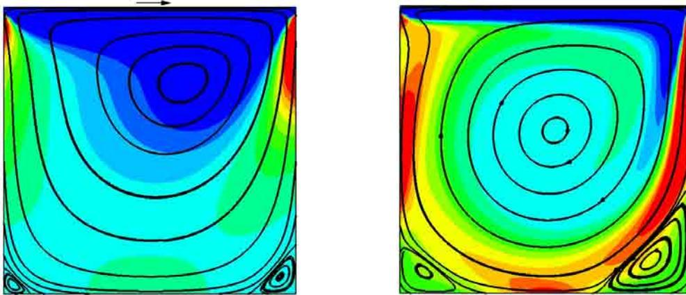
Figure 2. Streamlines on vorticity fields (+: red and -: blue). Left:  $Re = 100$ ; right:  $Re = 1000$ .
