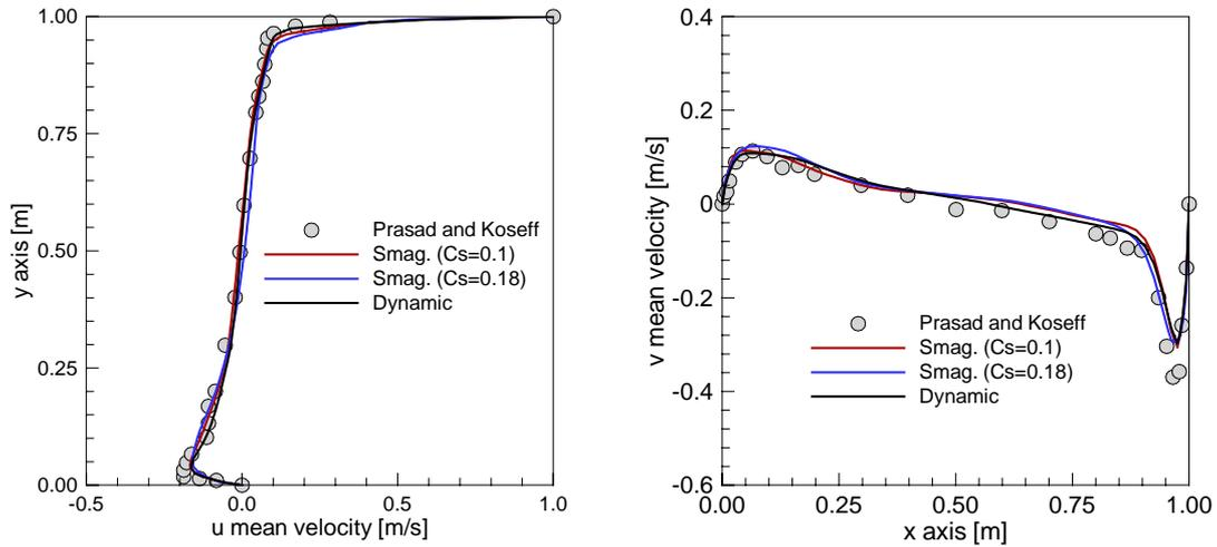
Figure 6. Comparison of the mean velocity at  $Re = 10000$ . Left: horizontal velocity; right: vertical velocity.
