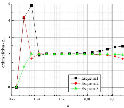
Figura 4.7.  $p_E$  de  $q_I$  do problema 1
