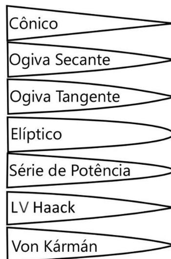
Figura 1.2 – Tipos de narizes de foguete. Adaptado <https://www.instructables.com/Design-a-Rocket-Nose-Cone-with-Software>
