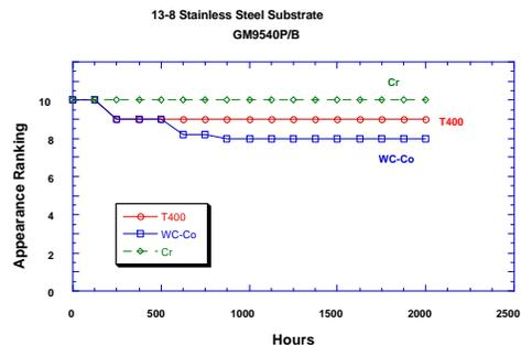
Figure 7. Appearance rankings for coatings on PH13-8Mo stainless steel substrates subjected to GM cyclic test
