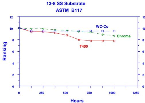
Figure 4. Appearance rankings for various coatings on the PH13-8Mo stainless steel specimens subjected to B117 salt fog test
