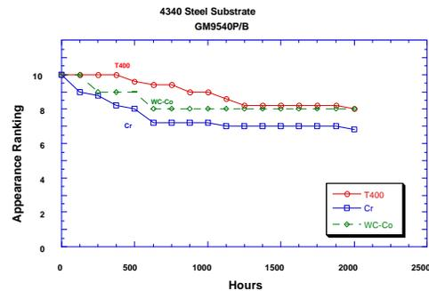
Figure 6. Appearance rankings for coatings on 4340 steel substrates subjected to GM cyclic test.
