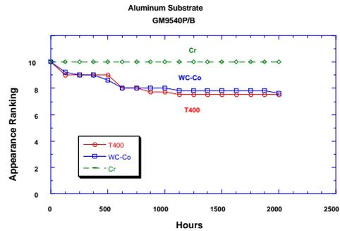
Figure 5. Appearance rankings for coatings on 7075 Al alloy substrates subjected to GM cyclic test.
