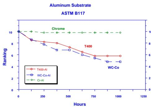
Figure 2. Appearance rankings for various coatings on the 7075 aluminum alloy specimens subjected to the B117 salt fog test
