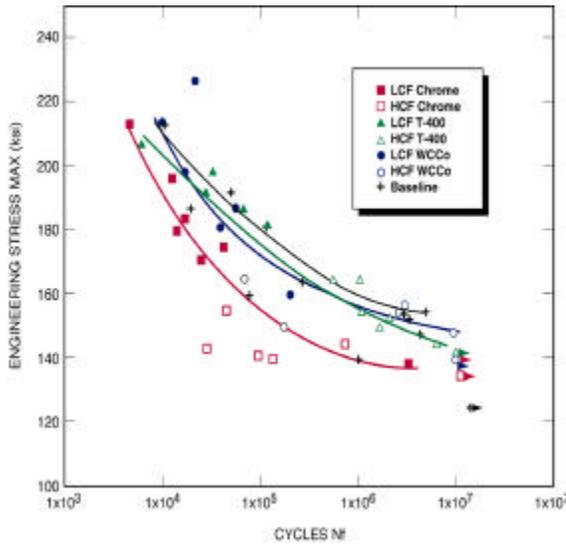
Figure 1. S/N data for smooth bar uncoated 4340 steel specimens and 4340 specimens coated with hard-chrome, HVOF WC/17%Co, and HVOF Tribaloy 400.
