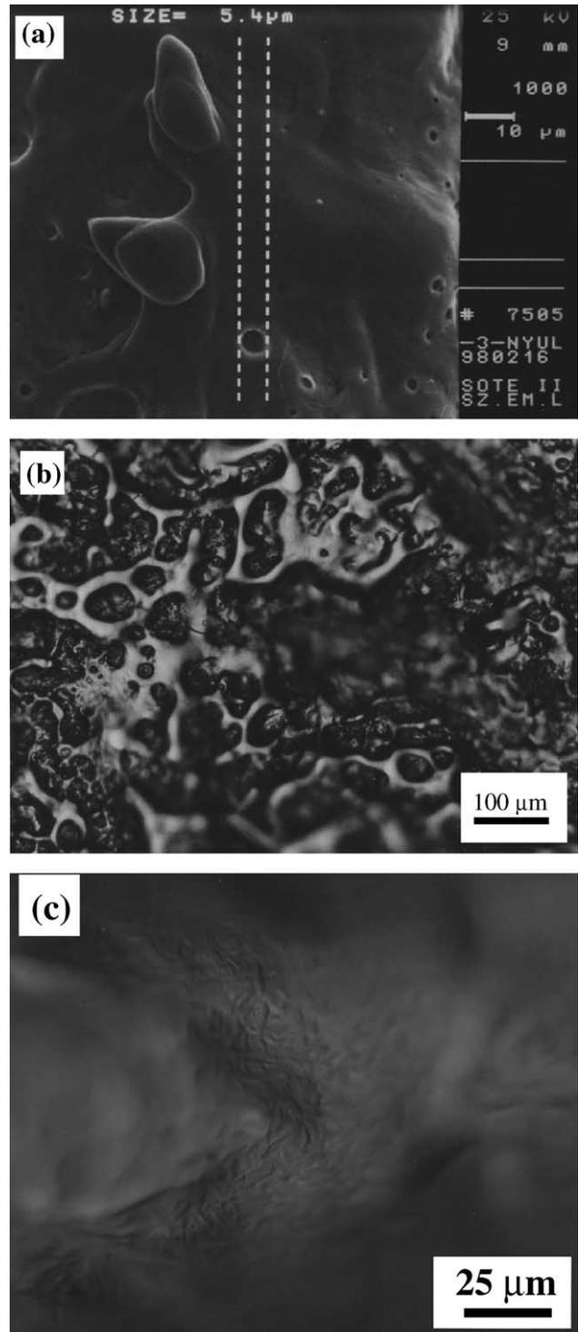
Fig. 4. Surface morphology of an  $\text{Al}_2\text{O}_3$  sand blasted and 3 J laser irradiated titanium implant surface by SEM 1000 $\times$  magnification (a) and by optical microscope 100 $\times$  magnification (b), and 400 $\times$  magnification (c).
