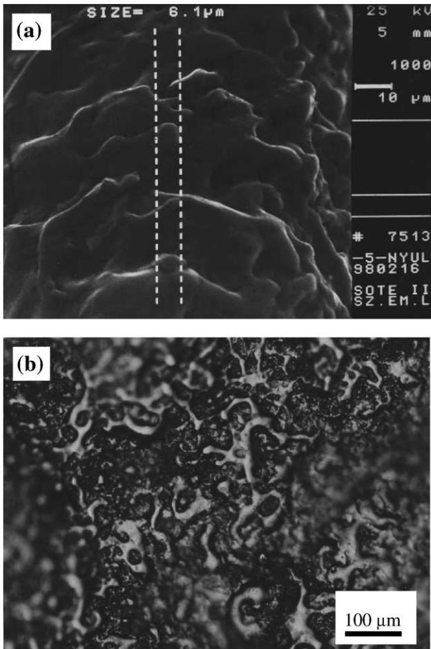
Fig. 3. Surface morphology of an  $\text{Al}_2\text{O}_3$  sand blasted and 1 J laser irradiated titanium implant surface by SEM 1000 $\times$  magnification (a) and by optical microscope 100 $\times$  magnification (b).
