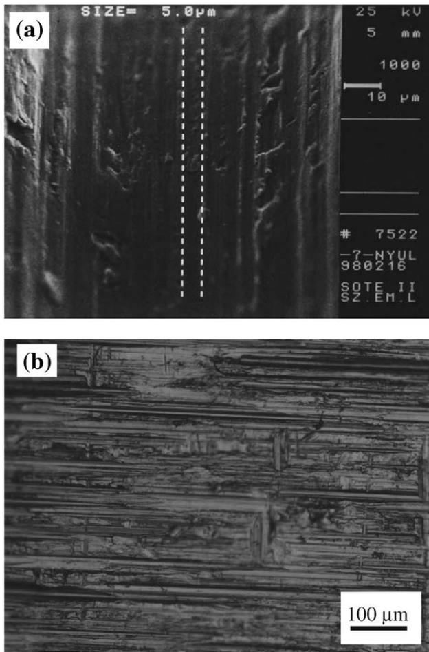
Fig. 1. Surface morphology of a machined titanium implant surface by SEM 1000  $\times$  magnification (a) and by optical microscope 100  $\times$  magnification (b).
