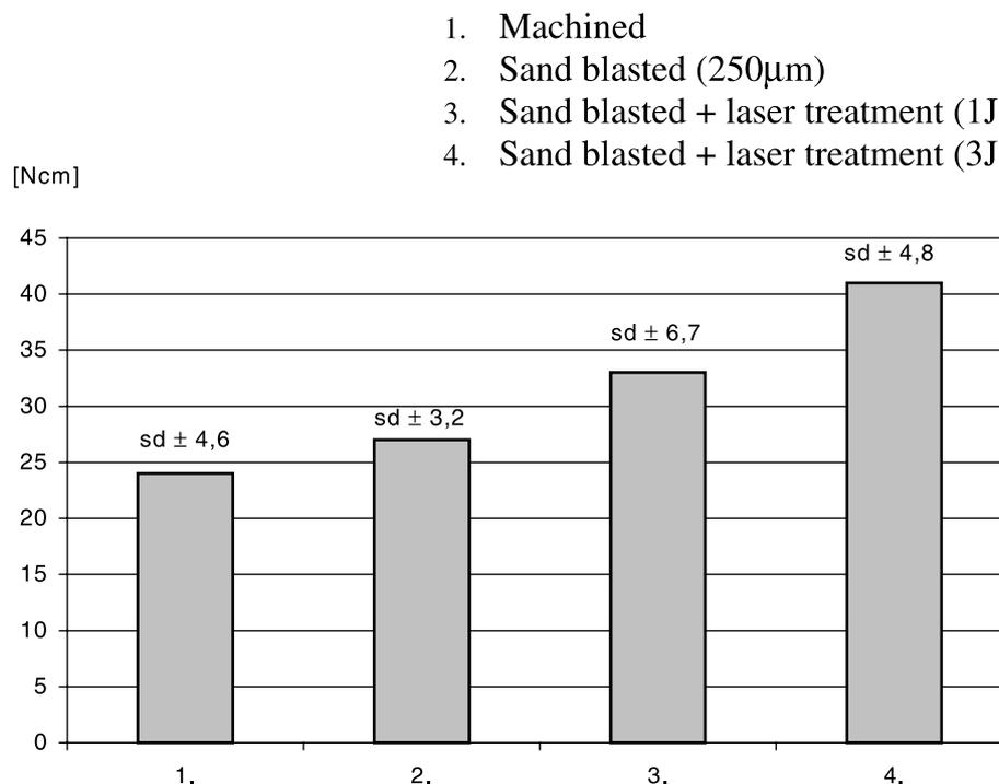
Fig. 5. Removal torque [N cm] data of different surfaces.
