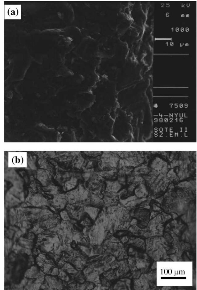
Fig. 2. Surface morphology of an  $\text{Al}_2\text{O}_3$  sand blasted titanium implant surface by SEM 1000  $\times$  magnification (a) and by optical microscope 100  $\times$  magnification (b).
