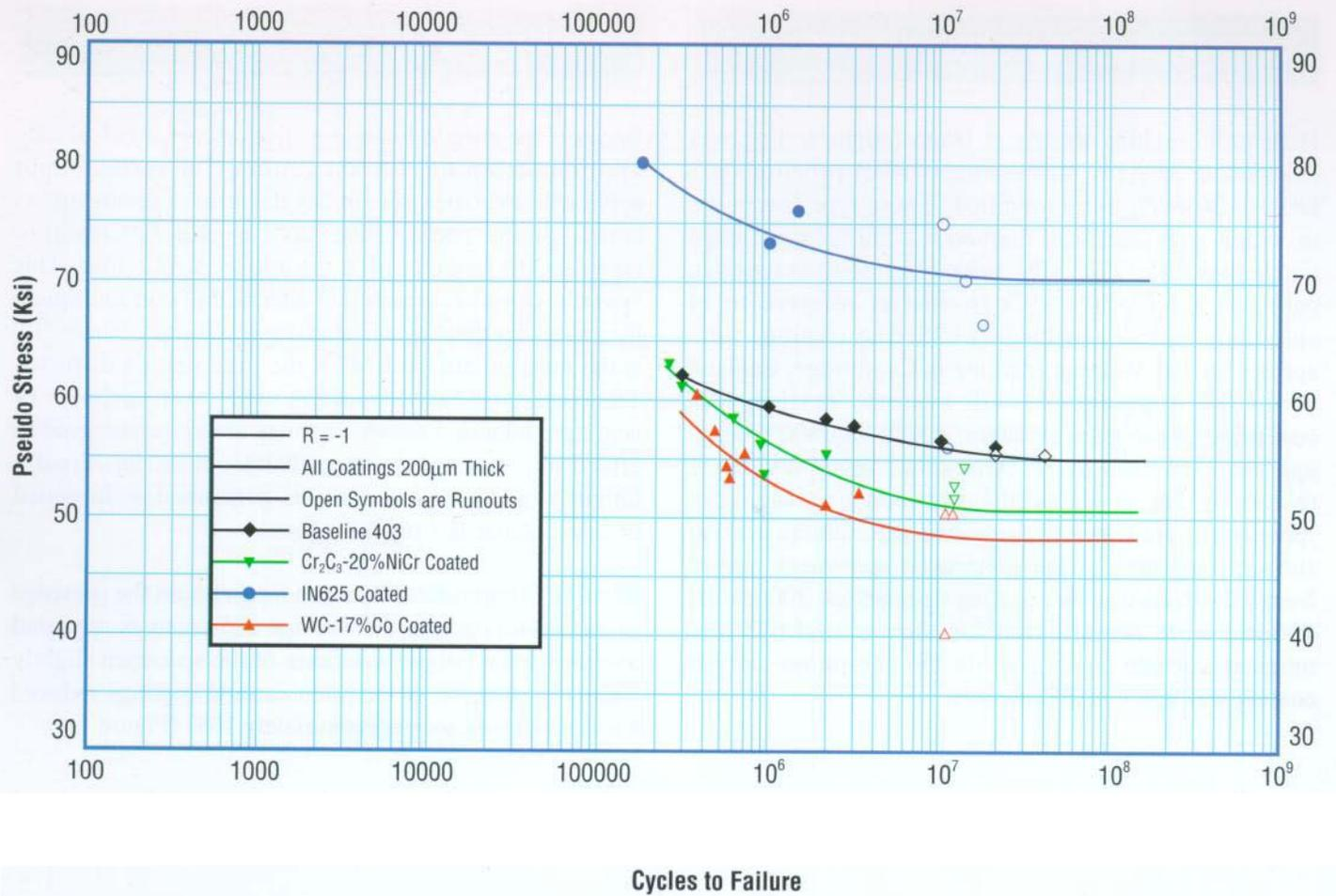
Figure 2. Effect of HVOF Coatings on the Fatigue Behavior of 403 Stainless Steel at 400°F
