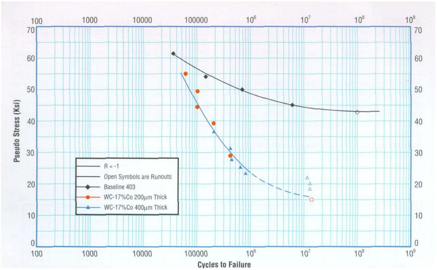
**Figure 5.** Effect of HVOF Tungsten Carbide Coating Thickness on the Fatigue Behavior of 403 Stainless Steel at 800°F
