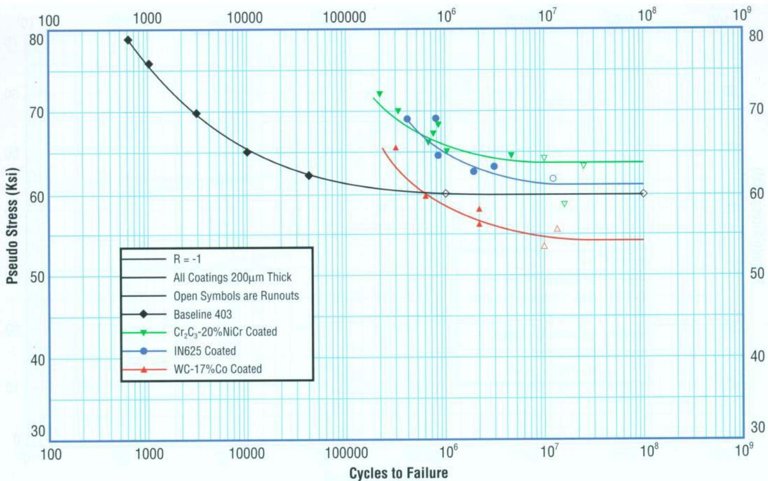
Figure 1. Effect of HVOF Coatings on the Room Temperature Fatigue Behavior of AISI 403 Stainless Steel
