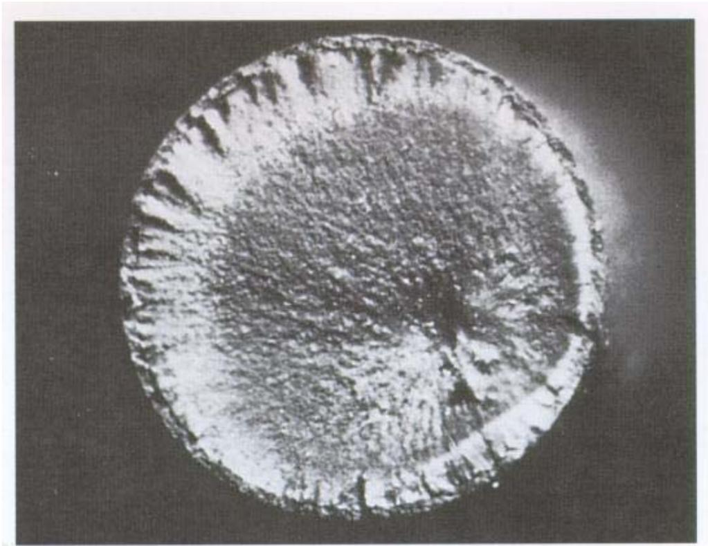
*Figure 8-15X. Photograph of fracture surface of tungsten carbide coated specimen tested at 800°F showing multiple origins.*
