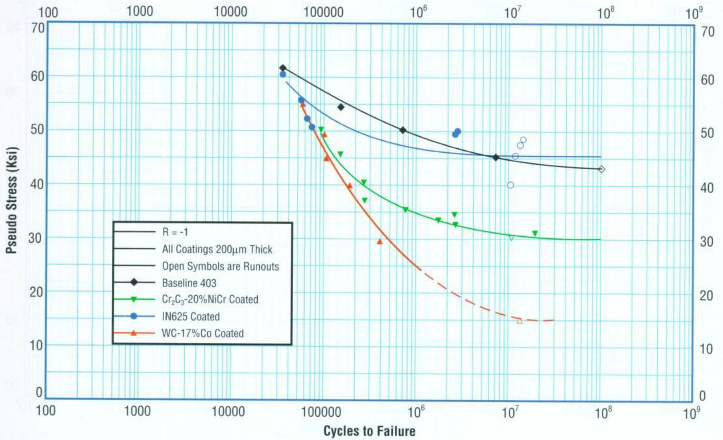
Figure 3. Effect of HVOF Coatings on the Fatigue Behavior of 403 Stainless Steel at 800°F
