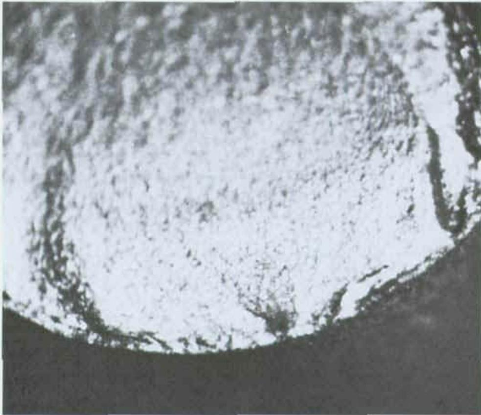
*Figure 6-15X. Photograph of fracture surface of an IN625 coated specimen tested at room temperature showing origin area.*
