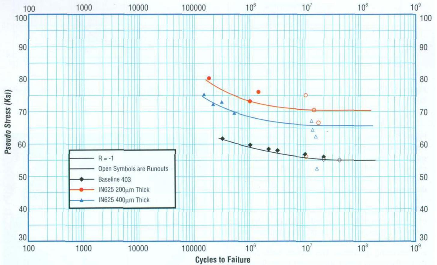
Figure 4. Effect of HVOF IN625 Coating Thickness on the Fatigue Behavior of 403 Stainless Steel at 400°F
