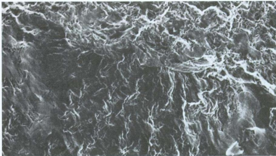
*Figure 9-51X. Scanning electron microscope photograph of fracture surface of chromium carbide coated specimen tested at 400°F showing delamination along coating/substrate interface.*
