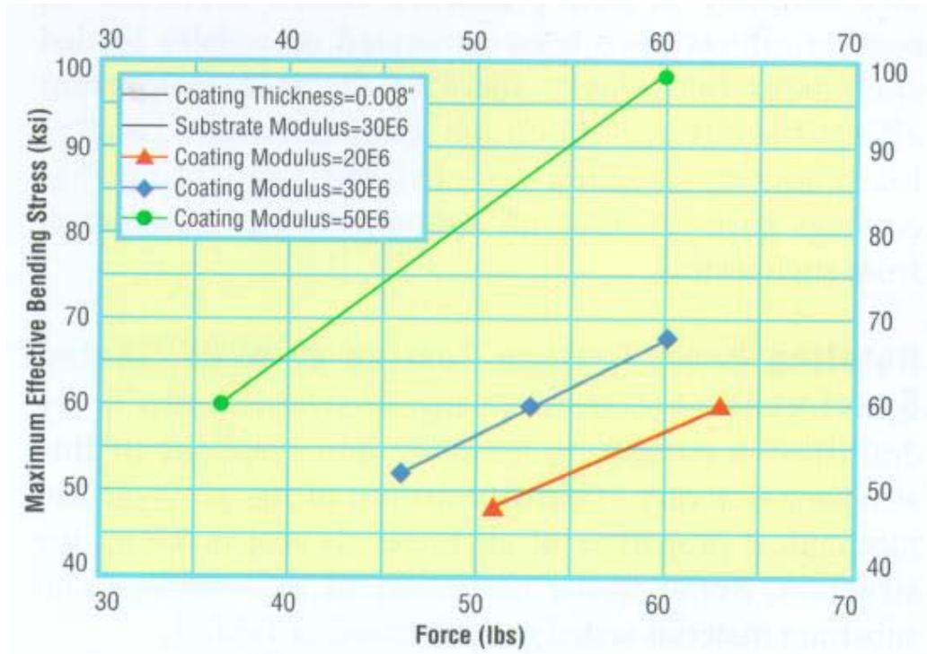
*Figure 10. Effect of Elastic Modulus Mismatch on the Effective Bending Stress of Thermal Spray Coated Krouse Type Rotating Beam Fatigue Specimens at Room Temperature*
