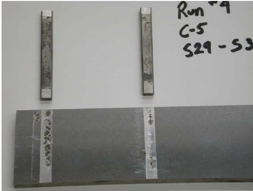
Figure 3-23. EHC Dithering in Contaminated Oil With Steel Counter-faces
