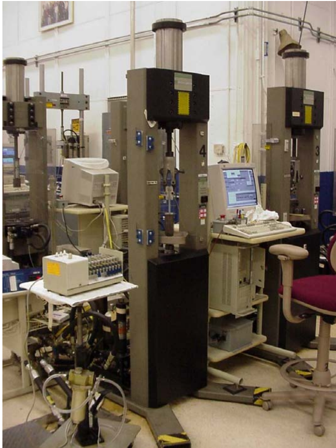
22,000 pound servo-hydraulic fatigue test frame
