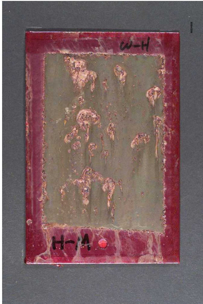
Figure 3-2. 0.001"-Thick WC/Co HVOF
