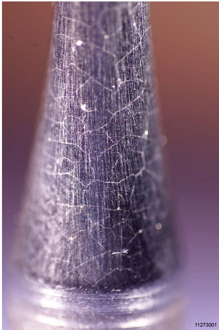
Figure 3-15. White Light of EHC Coated Specimen Showing Cracks Created By Machining Process
