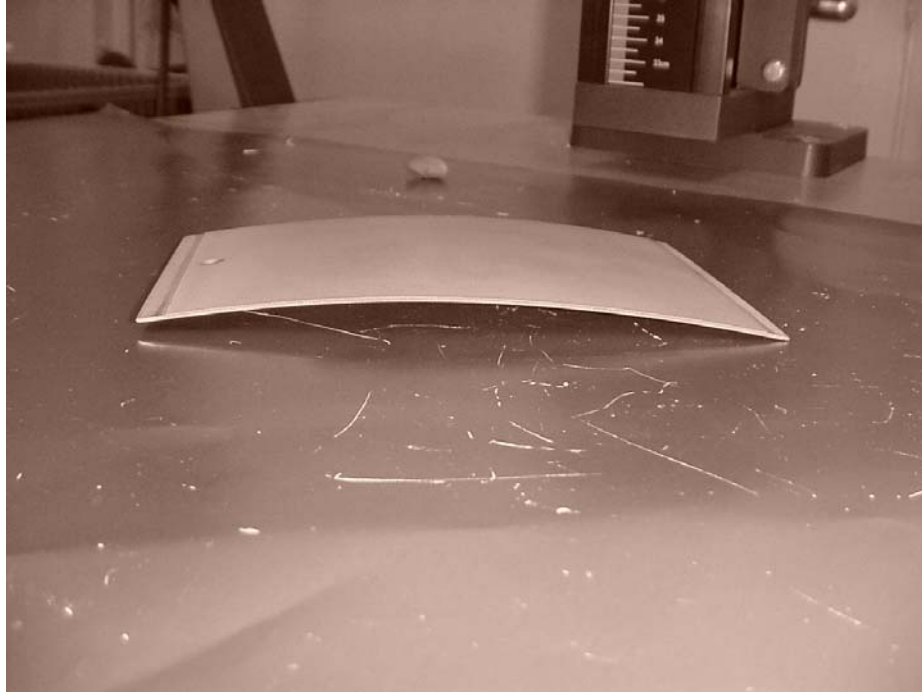
Figure 3-6. WC/Co Coated Panel, Top Surface Coated
