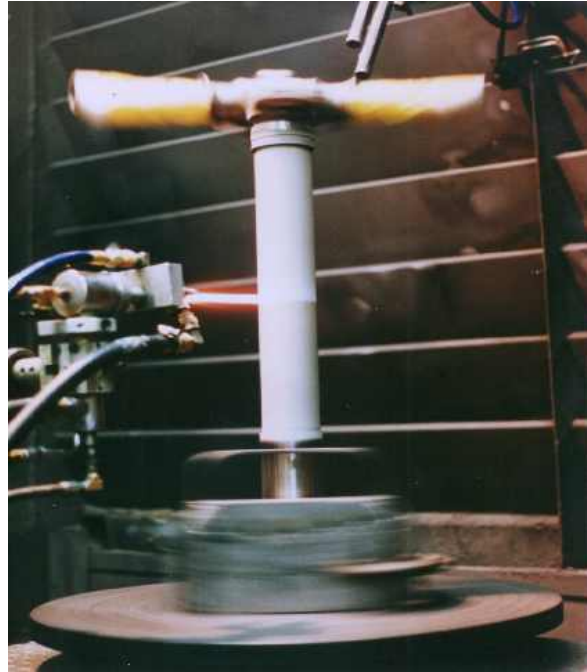
Figure 2-2. HVOF Spray of Landing Gear Inner Cylinder
