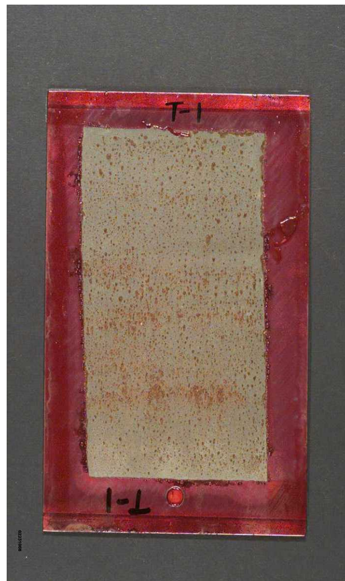
Figure 3-4. 0.001"-Thick Tribaloy T-800 HVOF
