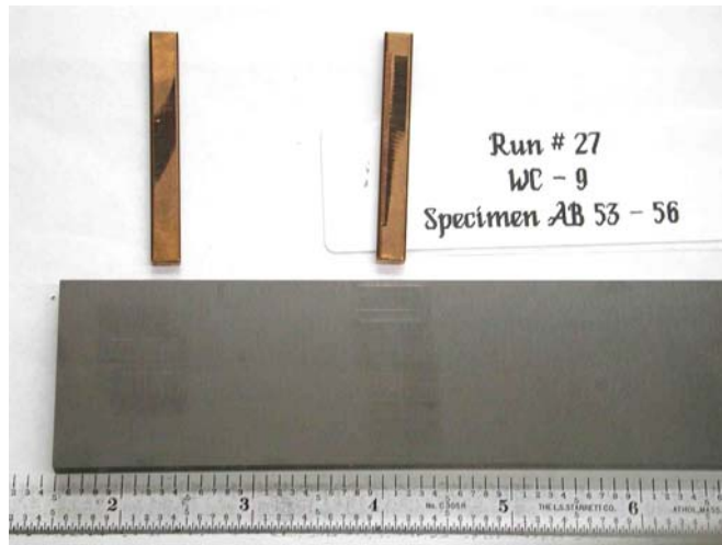
Figure 3-30. WC/Co Reciprocating Against Copper Counter-Faces
