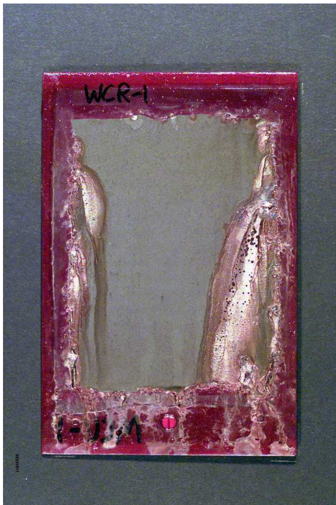
Figure 3-5. 0.001"-Thick WC/CoCr HVOF
