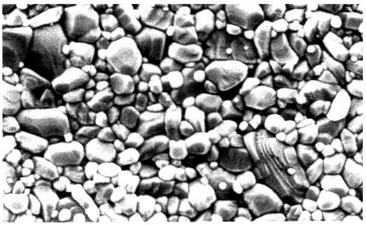
Figure 12.18 Microstructure of Hertel grade AC5 alumina/zirconia cutting ceramic, at 2500 times magnification.
