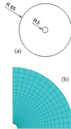
FIGURE 2. Samples for Hole Expansion (a) for experiments (b) quarter geometry for numerical simulation
