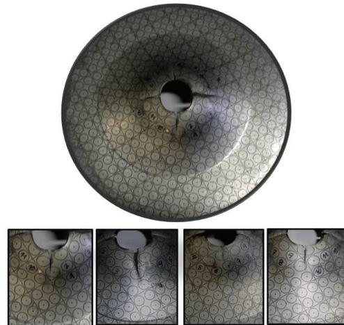
FIGURE 4. Deformed circles on HE sample
