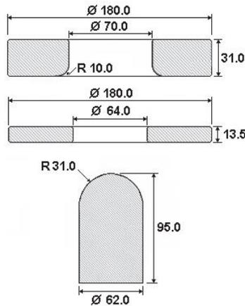
FIGURE 1. Experimental set-up for forming limit diagram
