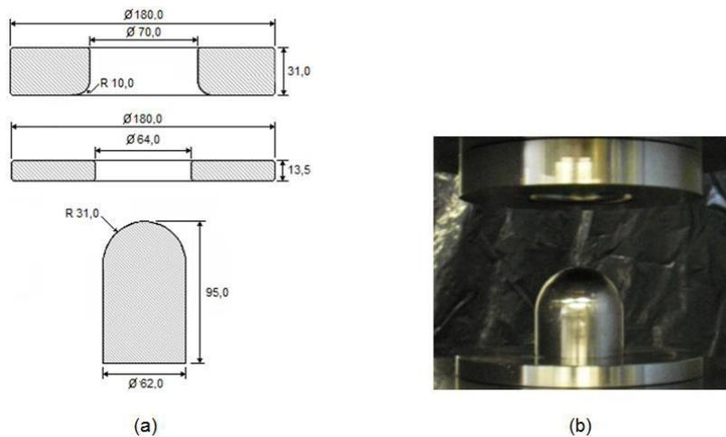
**Figure 1:** Tooling designed for implementation of Nakazima Tests.
