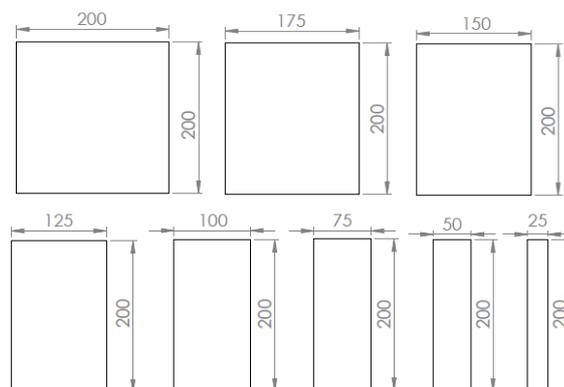
**Figure 2:** Specimens for implementation of Nakazima Tests (dimensions represented in mm).
