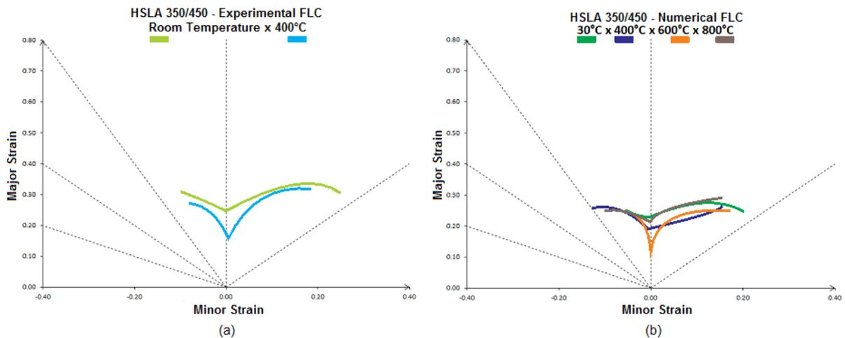
**Figure 4:** Experimental and numerical FLC for the HSLA 350/450 steel.
