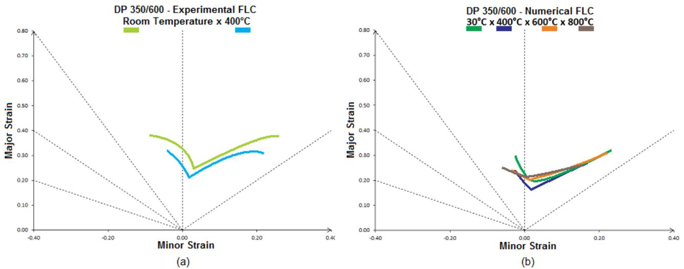
**Figure 5:** Experimental and numerical FLC for the DP 350/600 steel.
