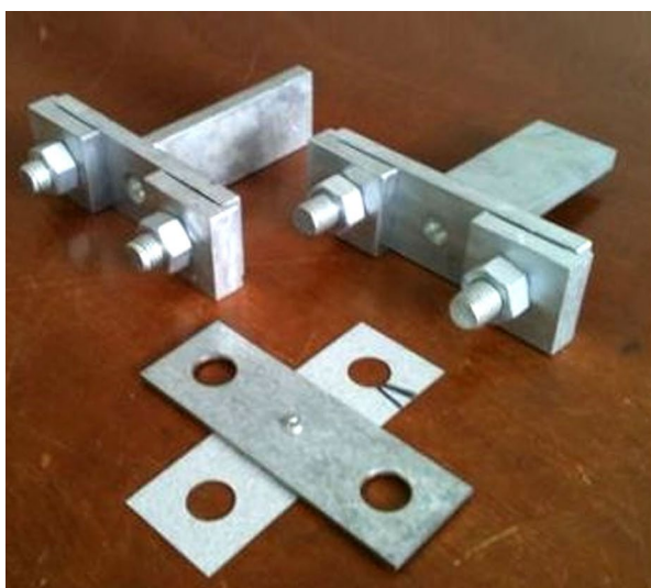
Fig. 5 Pull-out test: a test device and b proof sample
