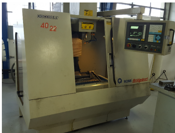
Figure 2. CNC vertical machining center.
