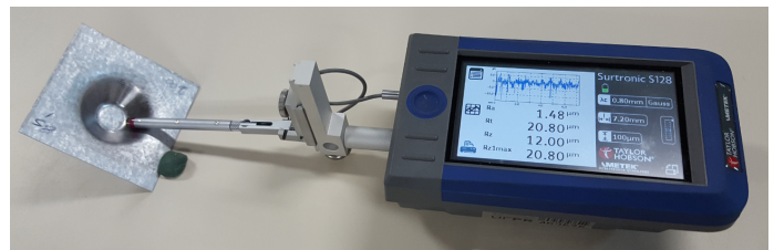
Figure 4. Taylor Robson roughness tester.
