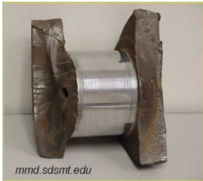
Failure of crankshaft journal
