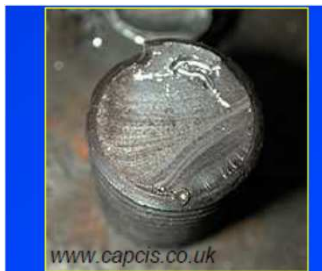
Fatigue failure of a bolt
