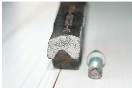
Fatigue failure of a bolt
