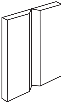
(C) VERTICAL WELDING TEST POSITION 3G
