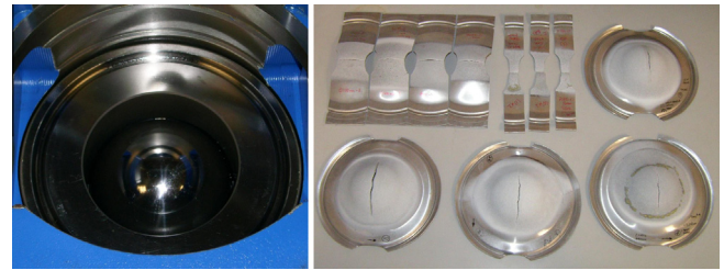
Fig. 4. Hemispherical punch and specimens used in the Nakazima tests.
