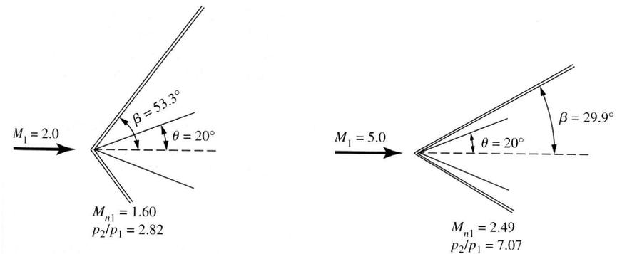
Figure 9.12 Effects of increasing the upstream Mach number.
