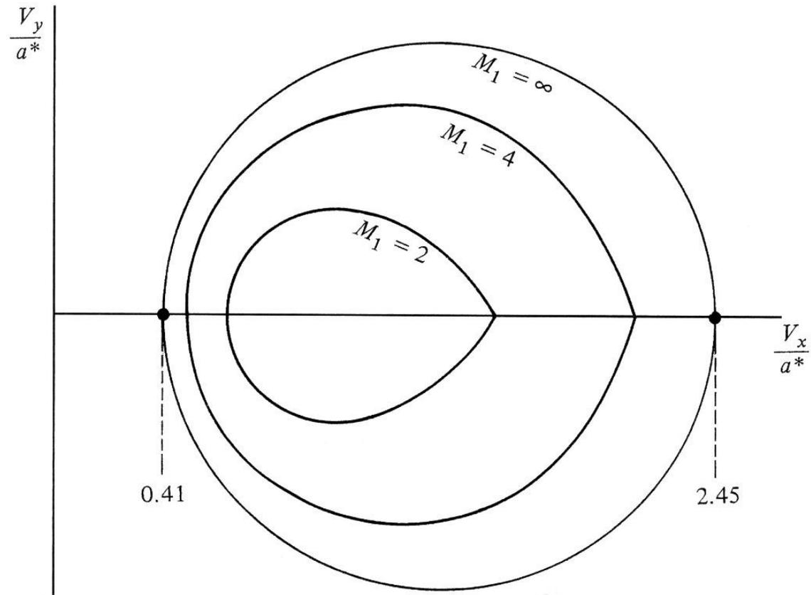
**Figure 4.17** | Shock polars for different Mach numbers.
