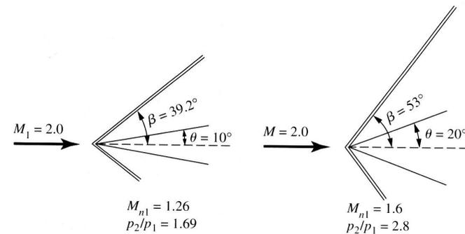
Figure 9.13 Effect of increasing the deflection angle.
