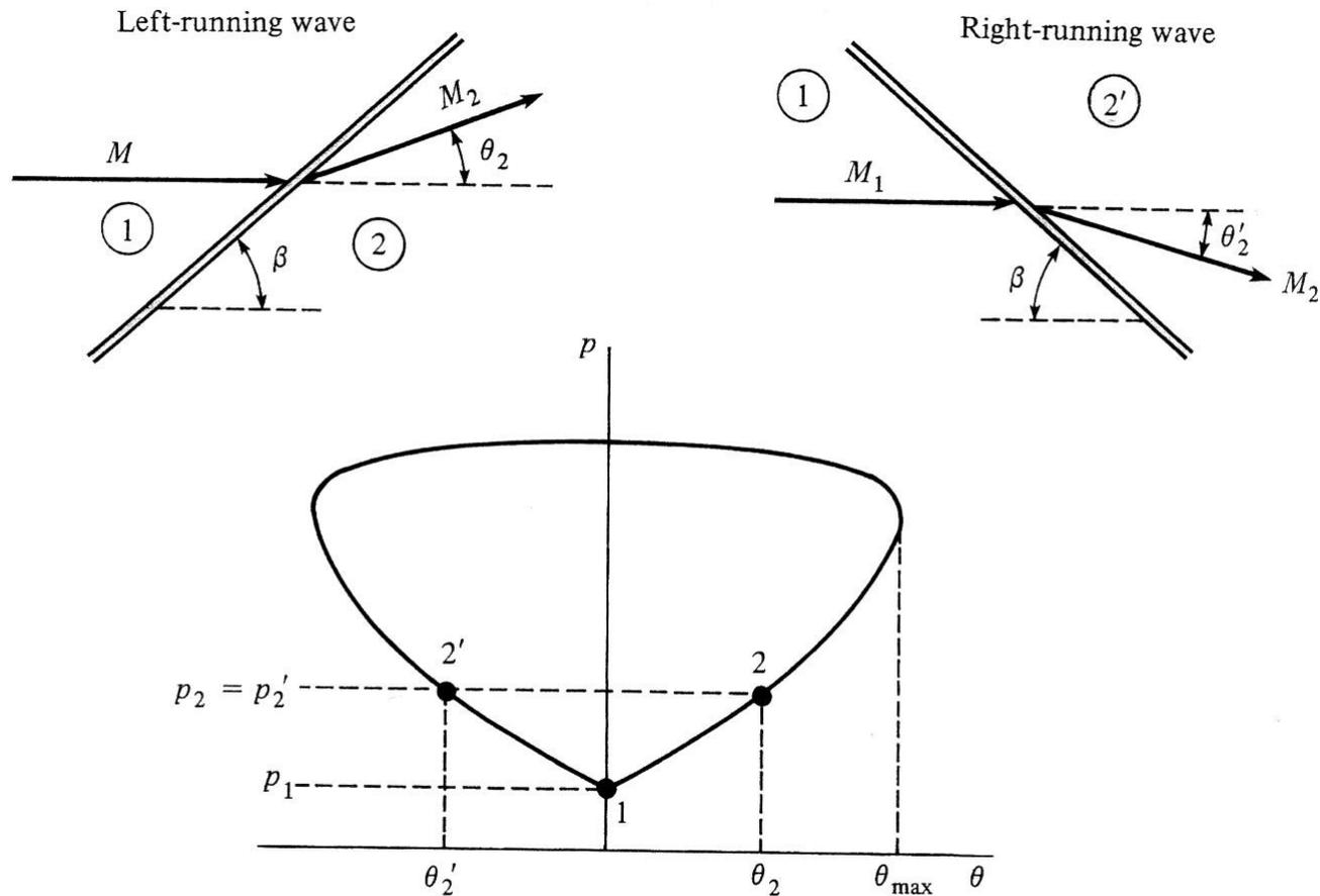
Figure 4.21 | Pressure-deflection diagram for a given  $M_1$ .
