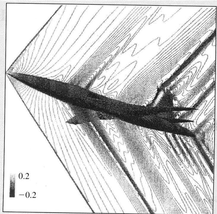
**Figure 9.1** Wave pattern on a supersonic transport configuration (without nacelles) at Mach 1.7. Computational fluid dynamic calculations by Y. Makino, et al., "Nonaxisymmetrical Fuselage Shape Modification for Drag Reduction of Low-Sonic-Boom Airplane," *AIAA Journal*, vol. 41, no. 8, August 2003, p. 1415.
