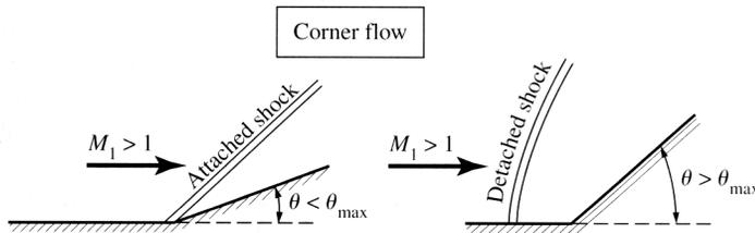
Figure 9.10 Attached and detached shocks.
