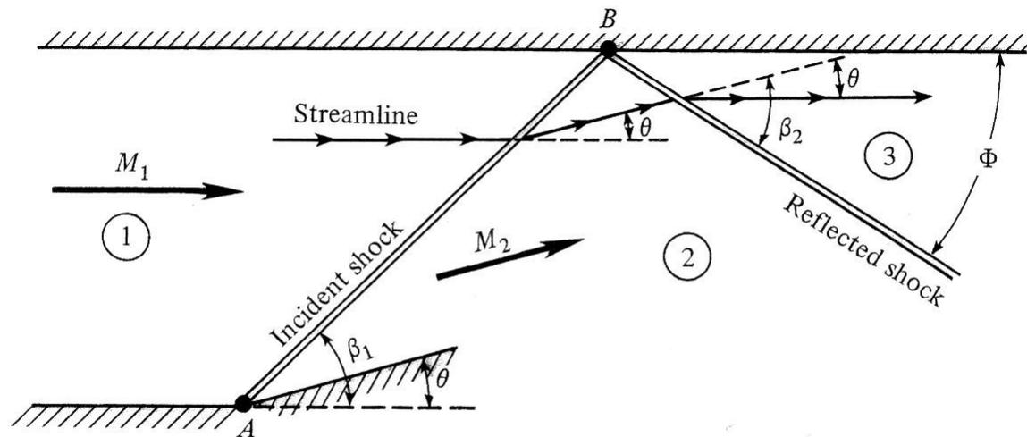
Figure 4.18 | Regular reflection from a solid boundary.
