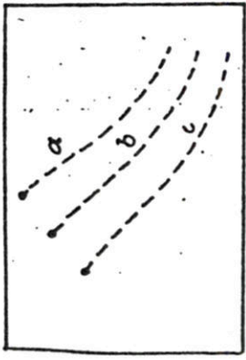
Fig. 1.8. Effect of particle size and opening diameters of the flow device on the flow of powders a) small opening dia. b) medium opening dia. c) large opening dia.
