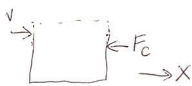
$$\frac{\partial M}{\partial t} - p(V-U)A = 0 \quad \therefore \quad \int_{M_0}^M dM = \int_0^t p(V-U)A dt \quad \text{onde } U = U(t)$$
