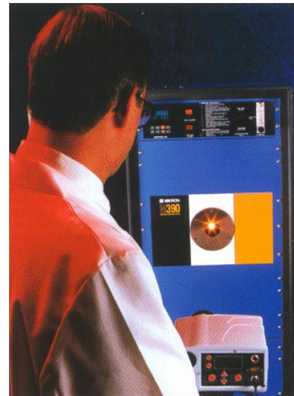
Operator calibrates a transfer standard (lower foreground)—an infrared thermometer with 0.1°C resolution—with a blackbody calibration source that provides temperatures from 600°C to 3000°C.
