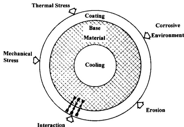
Fig. 1 Various factors encountered by thermal barrier coatings under service conditions (Ref 5)
