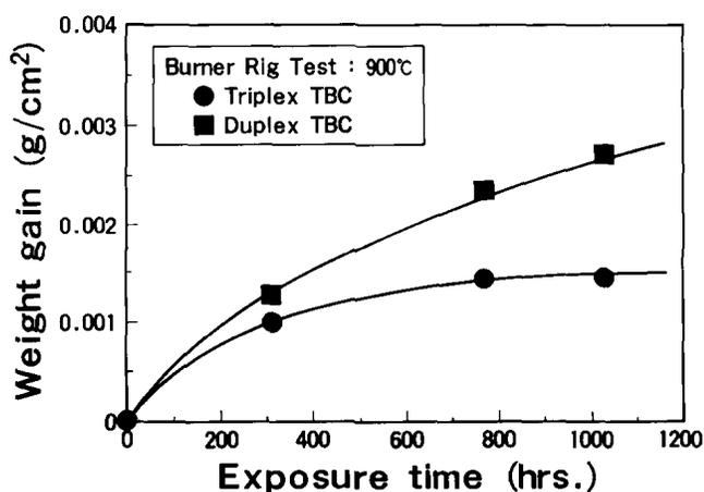
**Fig. 3** Weight gain of specimens in burner rig test. Test temperature: 900 °C
