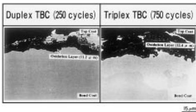
Fig. 6 Scanning electron microscopy images of cross section after the thermal cycle test
