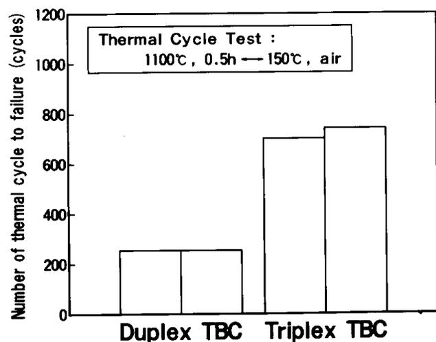
Fig. 5 Comparison of duplex and triplex thermal barrier coatings in a thermal cycle test
