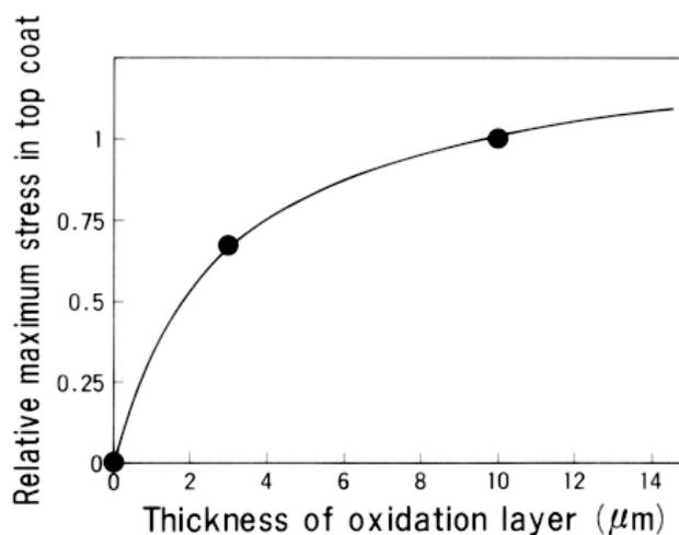
Fig. 9 Relation between maximum stress and thickness of oxidation layer
