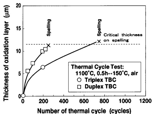
Fig. 10 Growth of oxidation layer in a thermal cycle test and critical thickness of spalling
