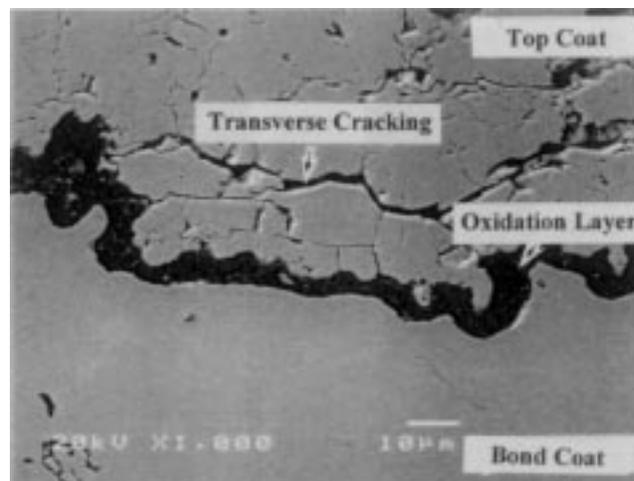
Fig. 7 Cracking in top coat before spalling. Thermal cycle: 100 cycles
