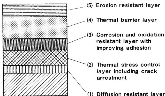
**Fig. 2** Concept of multilayered thermal barrier coating with different functions (Ref 6)
