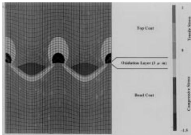
Fig. 8 Stress distribution occurred adjacent to uneven interface between bond coat and top coat
