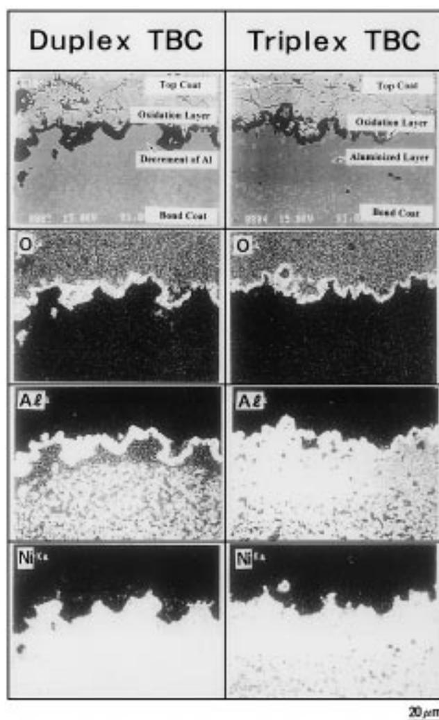
**Fig. 4** Scanning electron microscopy image and electron probe microanalyzer of a cross section after burner rig test. Bond coat/top coat: 900 °C, 1000 h
