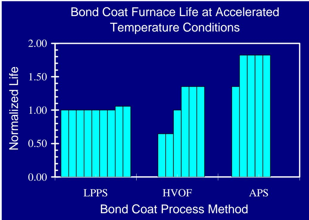
Figure 1. Normalized time to spallation under cyclic oxidation furnace test conditions.
