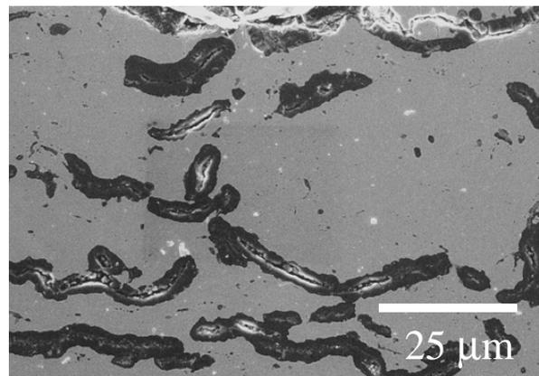
Figure 3. Internal oxidation along connected internal porosity boundaries within the APS bond coat.
