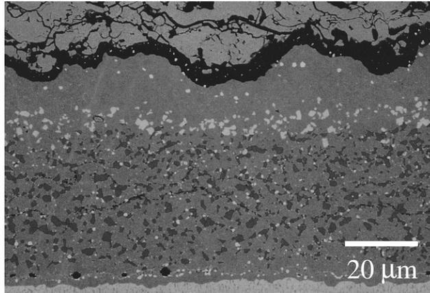
Figure 4. Third phase addition bond coat chemistry designed to reduce interdiffusion between the substrate and oxide.
