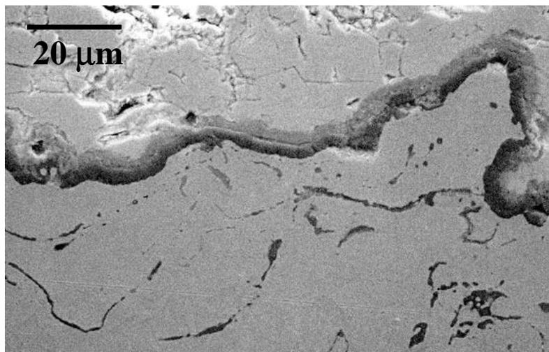
Figure 5. Deleterious reaction between the ceramic TBC and the protective alumina scale.
