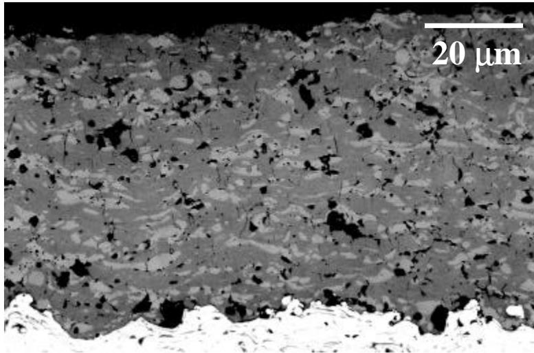
Figure 6. A multiphase coating resulting from plasma sprayed deposition of a single phase ceramic powder.
