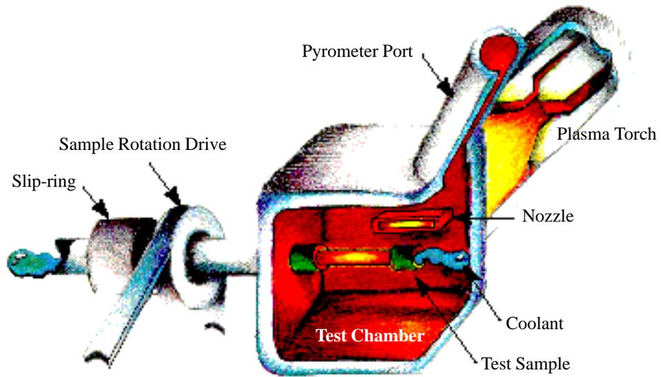
Figure 7. Schematic illustration of High Heat Flux Test Facility.
