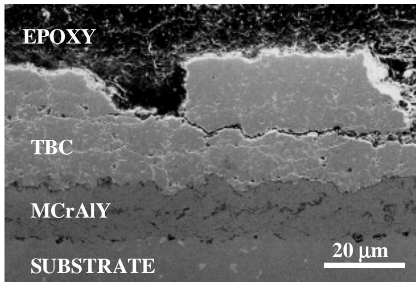
Figure 8. Spalled surface of an APS TBC.
