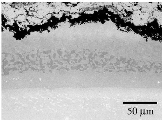
Figure 2. LPPS bond coat at failure.
