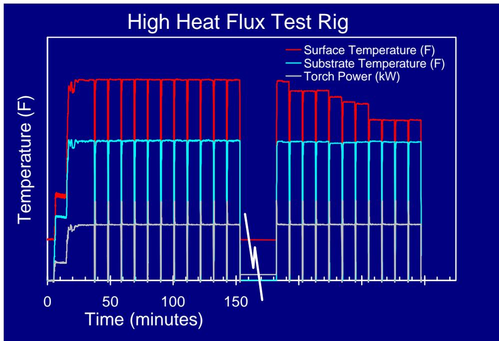
Figure 9. Characteristic time/temperature plot illustrating the stability and reproducibility of the plasma torch test. The decrease in surface temperature occurred as a result of layer spallation of the TBC.
