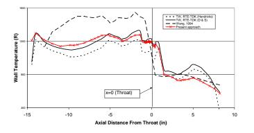
Figure 7: Hot-gas wall temperature comparison between the present approach and those of other methods for the SSME engine
