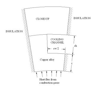
Figure 4: Configuration of one cell cooling channel
