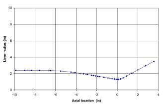
Figure 10: RP1-LO<sub>2</sub> rocket thrust chamber and nozzle contour showing station locations
