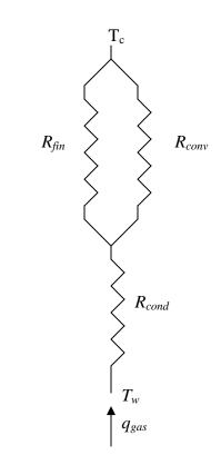
Figure 5: An equivalent thermal resistances for heat transfer in a regeneratively cooled rocket wall
