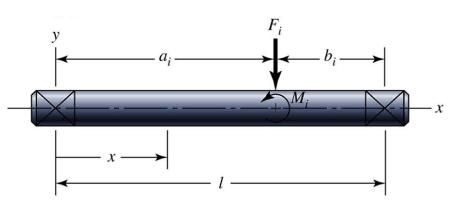
$$y_{AB} = \frac{F_i b_i x}{6EIL} (x^2 + b_i^2 - L^2) + \frac{M_i x}{6EIL} (x^2 + 3a_i^2 - 6a_i L + 2L^2)$$
