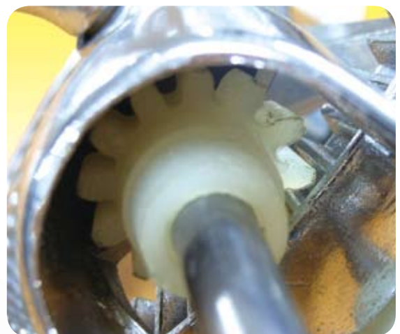
A gear to turn the mixer
