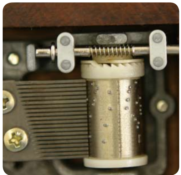
A musical movement (a worm gear pair is seen above.)
