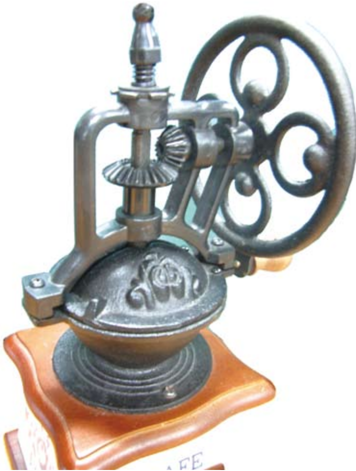
A pair of bevel gears to turn the mill
