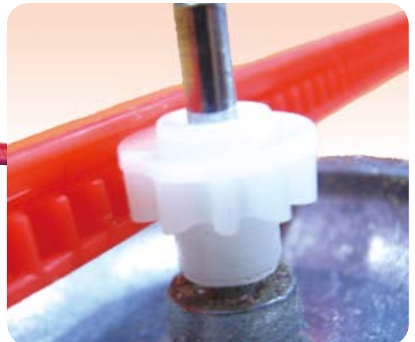
A belt-shaped rack and a gear to spin the top
