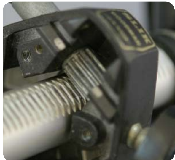
A round rack and a pinion
