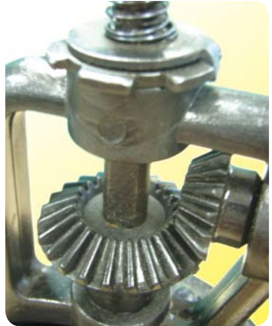
A pair of bevel gears to turn the mill
