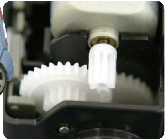
Gears transmitting power and motion to the tires.
