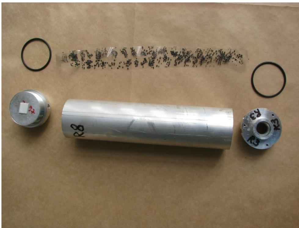
Motor-foguete Netuno-R-Beta: tubo-motor, tampa, tubeira, ignitor e 2 o-ring
