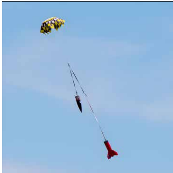
Figure 1: By knowing the drag coefficient of your parachute, you can accurately determine its descent rate.
