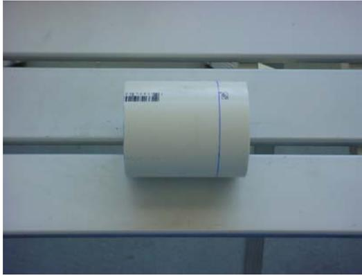
3. Using the hole template provided by Dan from Inverse Engineering, tape the template onto the 3" piece of PVC with the centerline of the holes aligned with the centerline that was drawn around the PVC.
