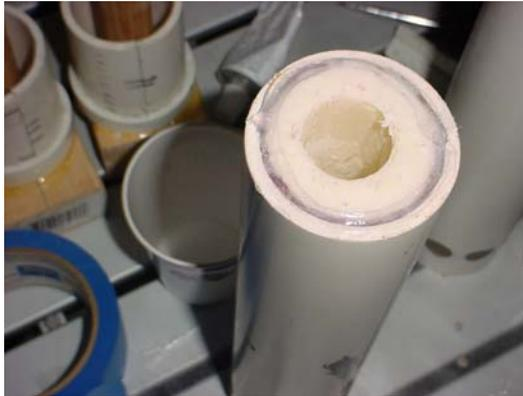
15. Using medium grey PVC cement, glue the 2" coupler/nozzle onto the 2" casing and let dry.
