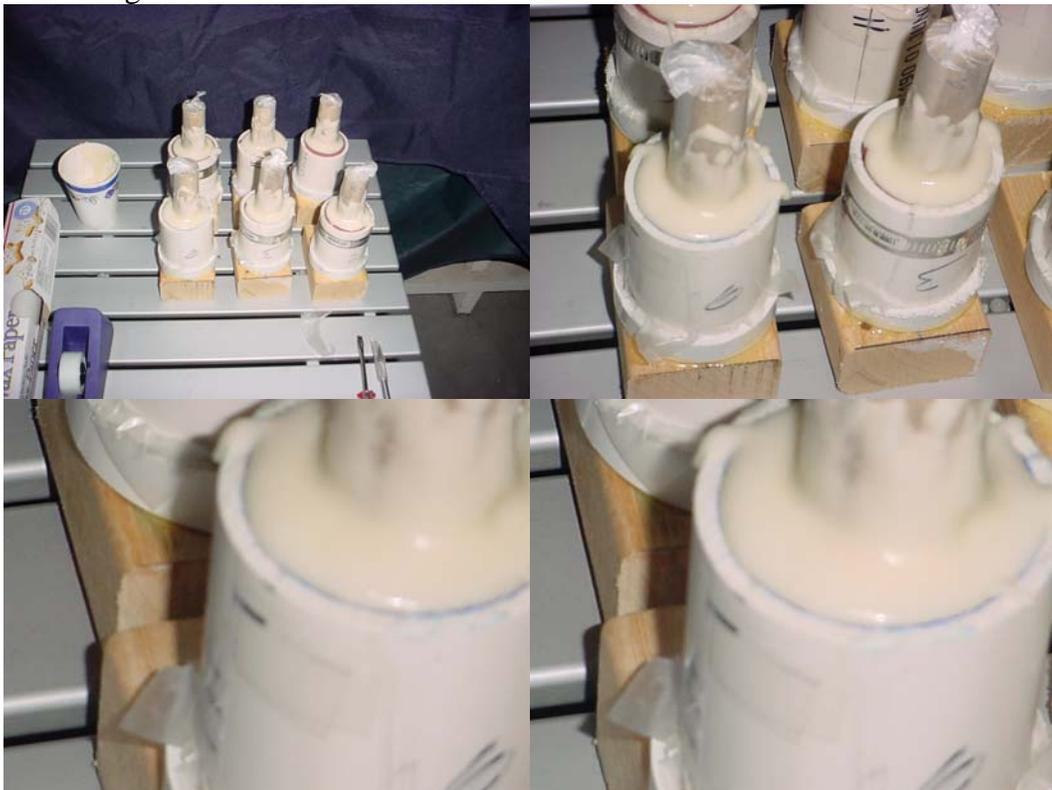
9. After about an hour, you will need to trim the top of the grains. If you do this while the propellant is still warm, it will be easier. Using a razor knife, trim off the excess propellant even with the top of the paper sleeve.
