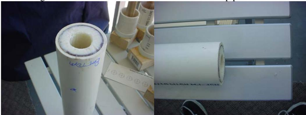
3. Cut a piece of 110 pound cardstock to cover the bore. This prevents the PourStone from entering the bore.
