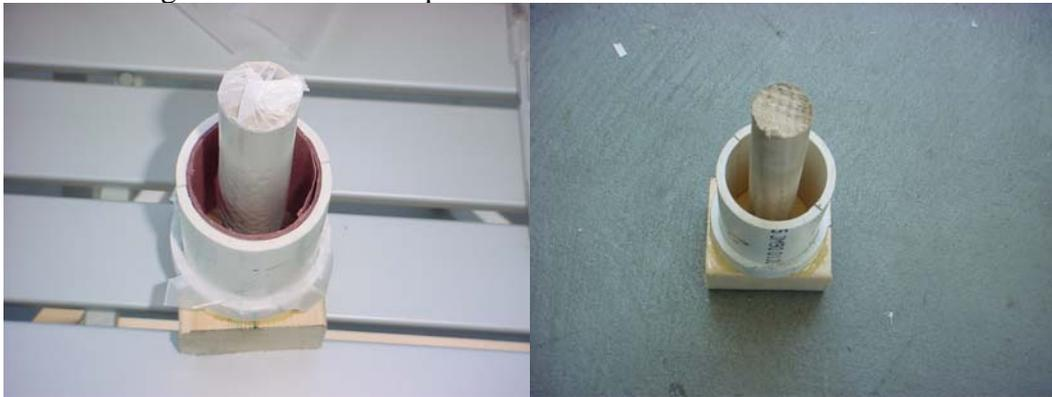
12. You need to make at least 3 of these casting fixtures in order to cast all 3 grains at the same time.
