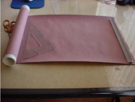
3. After test-fitting the paper around the pipe, insert the tube and PVC former into the 2" PVC pipe to make sure it fits. It should not be tight to push in, it should go in easily. If you have to force it in, it is too tight. Unroll a little bit at a time and cut off the excess and re-check the fit. After a satisfactory fit is achieved, unroll the paper all the way except for the last wrap.
