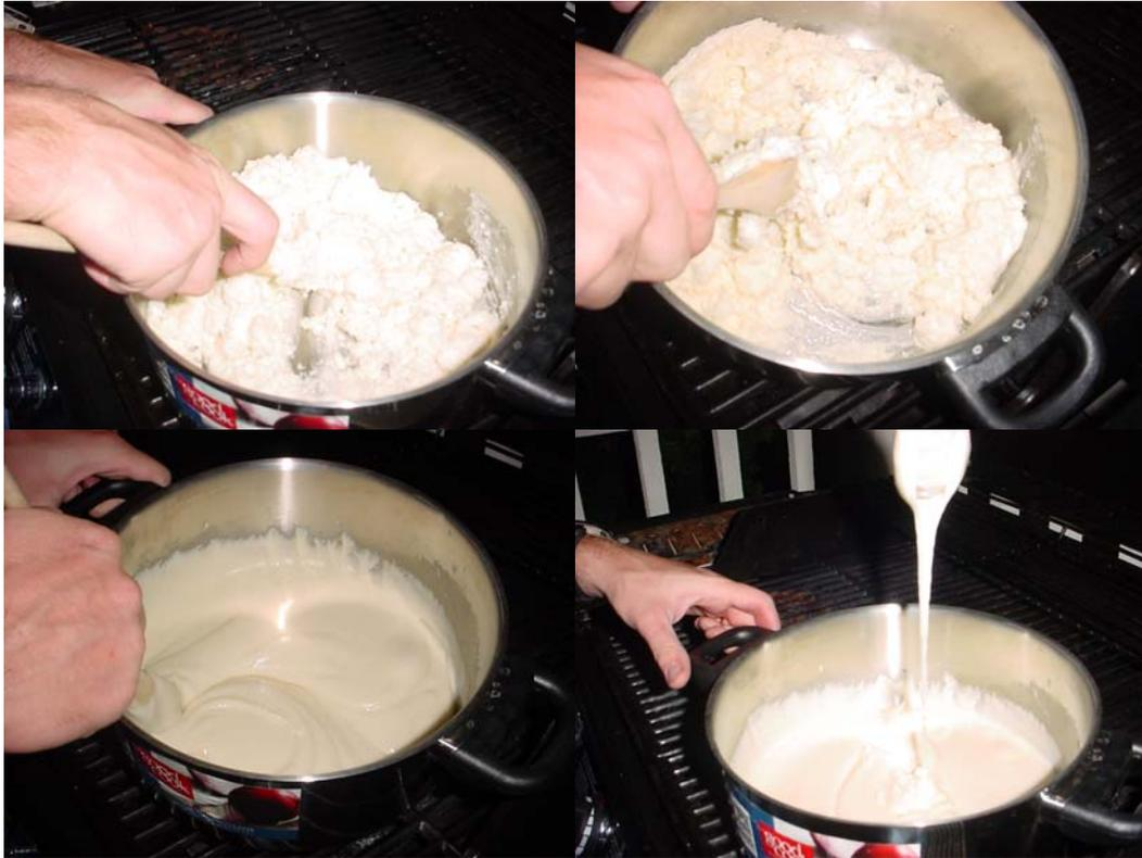
6. After the mixture is COMPLETELY melted, get one of the completed casting fixtures and scoop small amounts of propellant into the molds. This can be tricky until you get the hang of it. Fill the paper mold all the way to the top plus a little extra.
