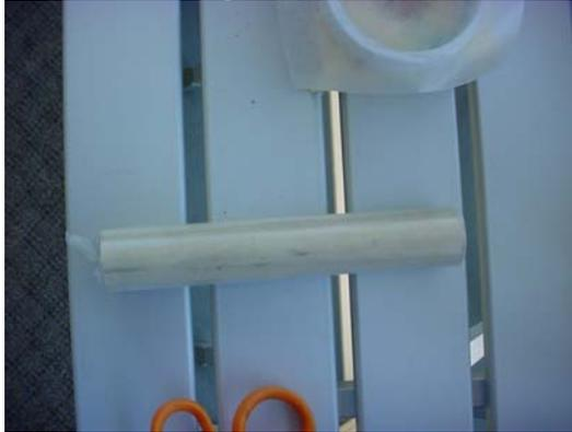
8. Place a piece of wax paper over the 2" coupling and press the cut PVC pipe over this until it is seated against the wood base.
