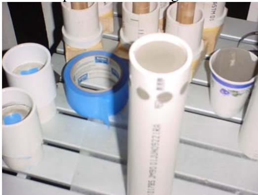
12. Inspect the “pins” that were created for any voids. If there is any, simply mix up more PourStone and fill in the voids and let it dry.
