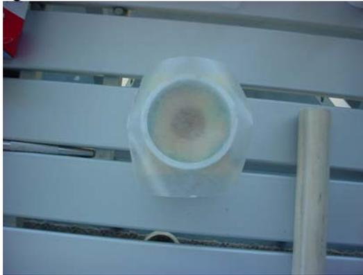
9. Using a razor knife, cut an "X" over the 1" hole in the base and inset the 1" bore rod into the hole.
