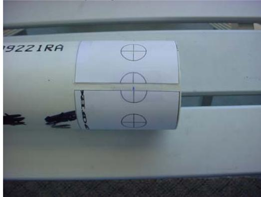
4. Drill the holes using a 5/8" Forstner bit and remove the template.
