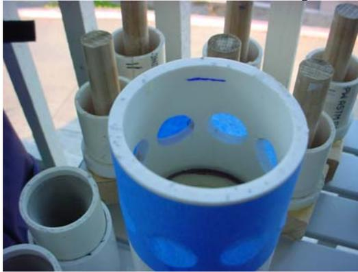
9. Mix up enough PourStone to fill the “TOP” of the motor case up to the mark that was drawn.
