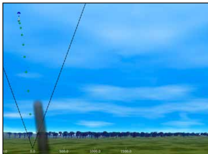
Figure 5 - The apogee of the flight stayed inside the weathercocking cone (black lines), indicating a nice straight-up flight.
