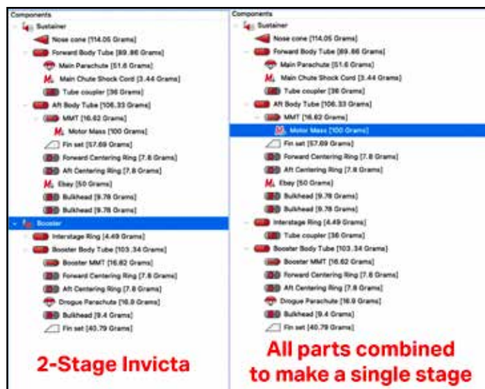
Figure 7 - The parts tree of the 2-stage Invicta (left side), and after the booster stages' parts were attached to the sustainer to make a single-stage version of the rocket.
