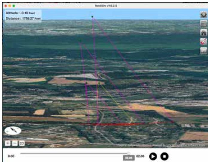
**Figure 13 - RockSim Pro will allow you to compare the trajectories of two simulations so you can pick the one that looks best to you.**
