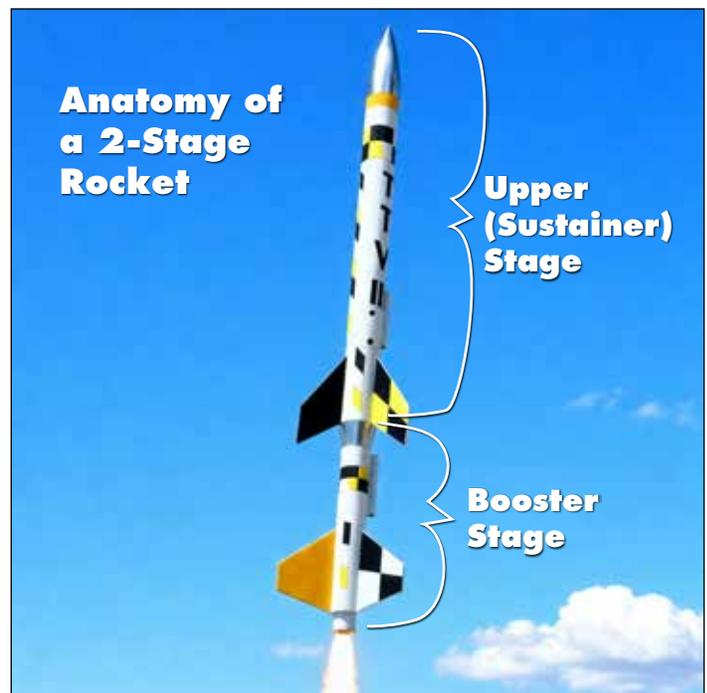
Figure 3 - Anatomy of a 2-stage rocket.
