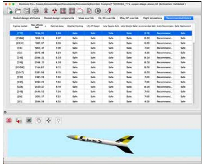
**Figure 12 -** The final list of motors to choose from for the upper stage. Sort the list by "Max. Altitude"
