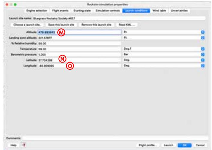
**Figure 10 - Also adjust the launch position of the rocket in the "Launch Conditions" tab, since it has moved up and off the launch pad.**
