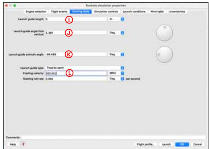
**Figure 9 - The "starting state" for the upper stage will be the position of the 2-stage rocket at the moment of staging.**
