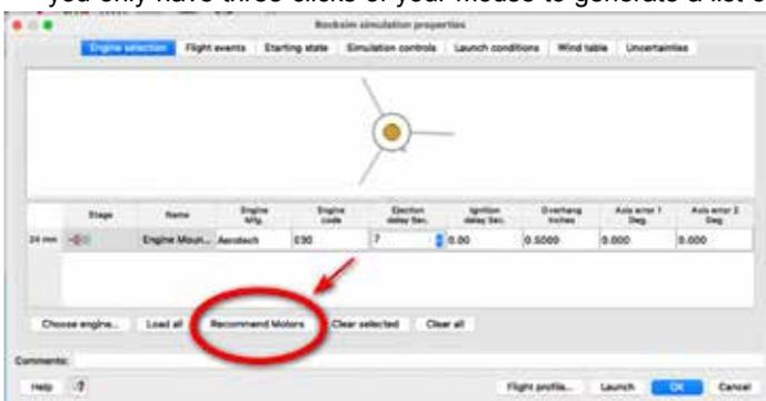
**Figure 7 - Click the "Recommend Motors" button to get an extensive list of motors that will work in your rocket.**
