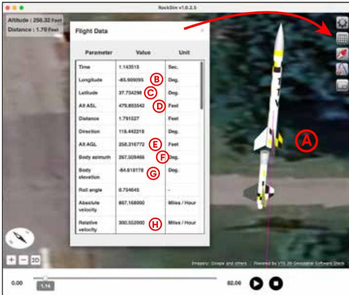
**Figure 8 - From the Launch Visualizer in RS-Pro, get the position of the rocket at the staging point in the flight.**
