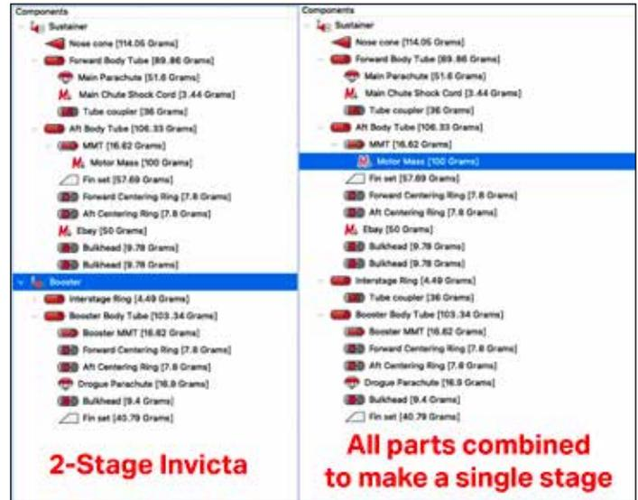
Figure 2 - To convert a two stage rocket, copy all the parts from the booster stage, and paste them to the bottom of the sustainer parts.
