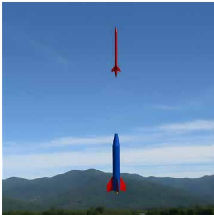
Figure 1: A "Boosted Dart" is a special 2-stage rocket that doesn't have a motor in the upper stage. The lower stage falls away due to drag-separation.
