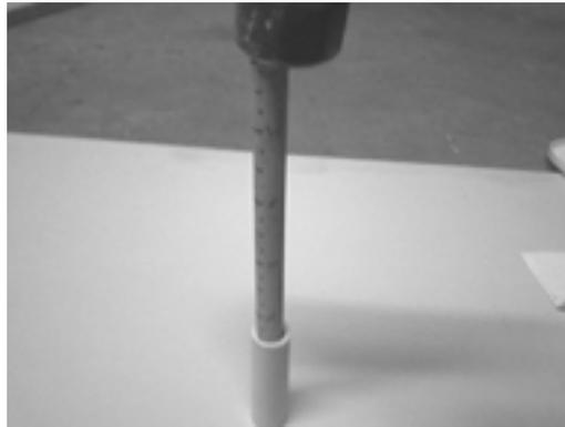
*Figure 8-5: Ramming the nozzle clay into the bottom of the tube with a ramming tool and hammer.*
