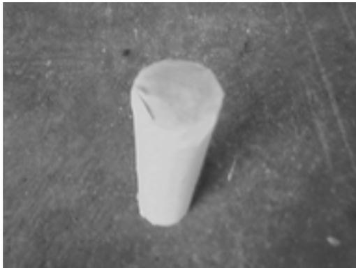
*Figure 12-5: Tape put over the black powder to hold it in place.*
