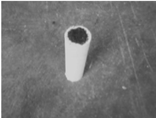
*Figure 12-4: Black powder scattered on the outside of the nozzle.*
