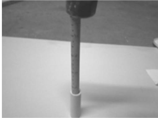
*Figure 8-8: Ramming the propellant into the bottom of the tube with a ramming tool and hammer.*
