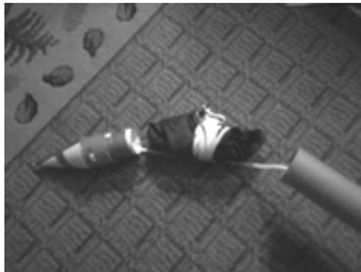
*Figure 16-22: Roll the parachute up so it can fit into the model rocket.*
