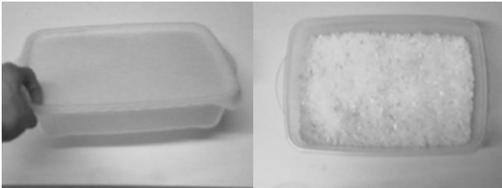
*Figure 19-2: An airtight container is used with salt in it for a desiccator.*
