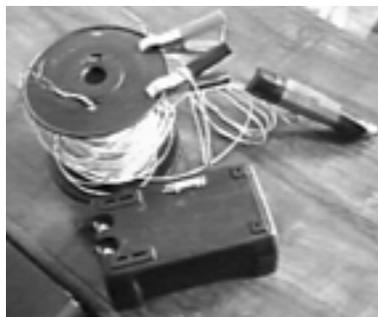
*Figure 14-2: An electrical ignition system.*
