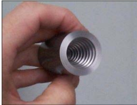
Step-drilled divergent passage of A-100M nozzle. A boring tool is then used to finish the contour.
