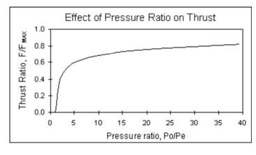
This chart plots the thrust ratio,  $F/F_{max}$ , to the pressure (or *expansion*) ratio, where  $F_{max}$  is the thrust that could be obtained with an infinite expansion ratio (i.e. expanding into a vacuum, with Pe=0). In the chart, the indicated thrust, F, excludes the pressure thrust term. The total thrust produced is given by  $F_{total} = F + (Pe-Pa)$  Ae.
