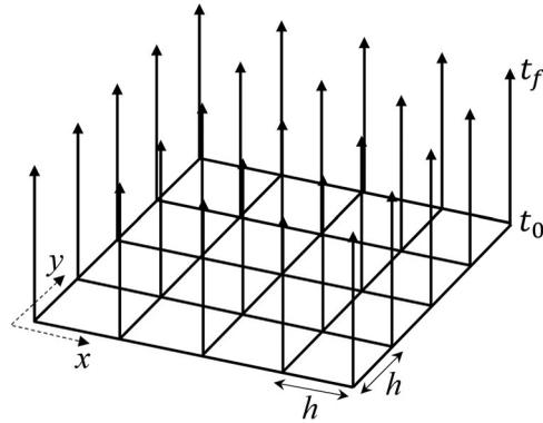
**Figure 2.** Waveform relaxation method scheme.
