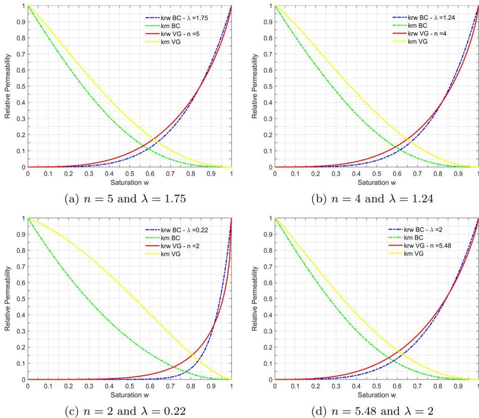
**Figure 5.** Curves of the relative permeabilities of the wetting and non-wetting phases for various  $n$  and  $\lambda$  parameters for VG and BC parameterizations.
