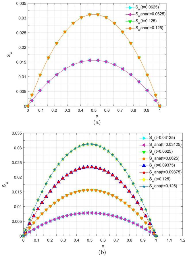
**Figure 6.** Numerical and analytical solutions for  $S_w$  using the VG parameterization with  $n = 5$  at different time steps for a mesh (a)  $N_x = N_t = 16$  and (b)  $N_x = N_t = 32$ .
