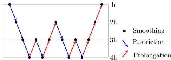
Figure 3. W-cycle for four mesh levels.
