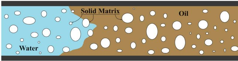
**Figure 1.** Illustration of a one-dimensional porous medium filled with two fluids, water and oil.
